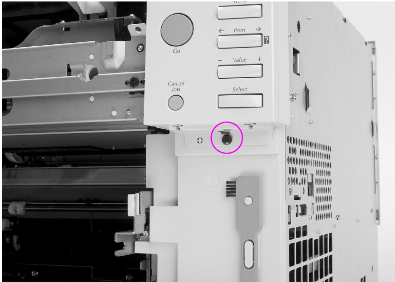
Figure 6-11 Control panel removal and replacement
