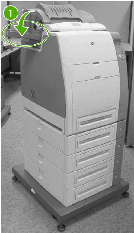
Figure 6-193 Remove the staple cartridge (1 of 2)
