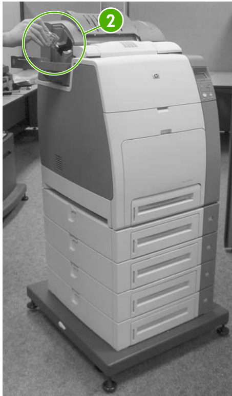
Figure 6-194 Remove the staple cartridge (2 of 2)
