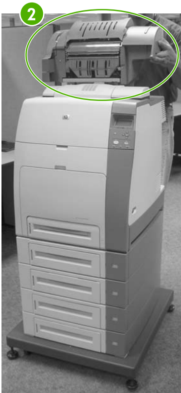
Figure 6-182 Remove the stapler/stacker from the printer (2 of 2)
