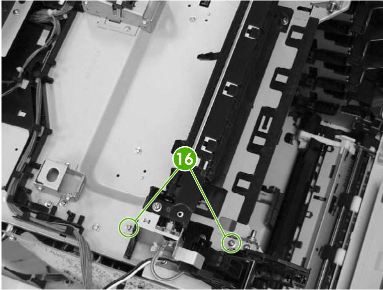
Figure 6-94 Remove the delivery assembly (8 of 9)
