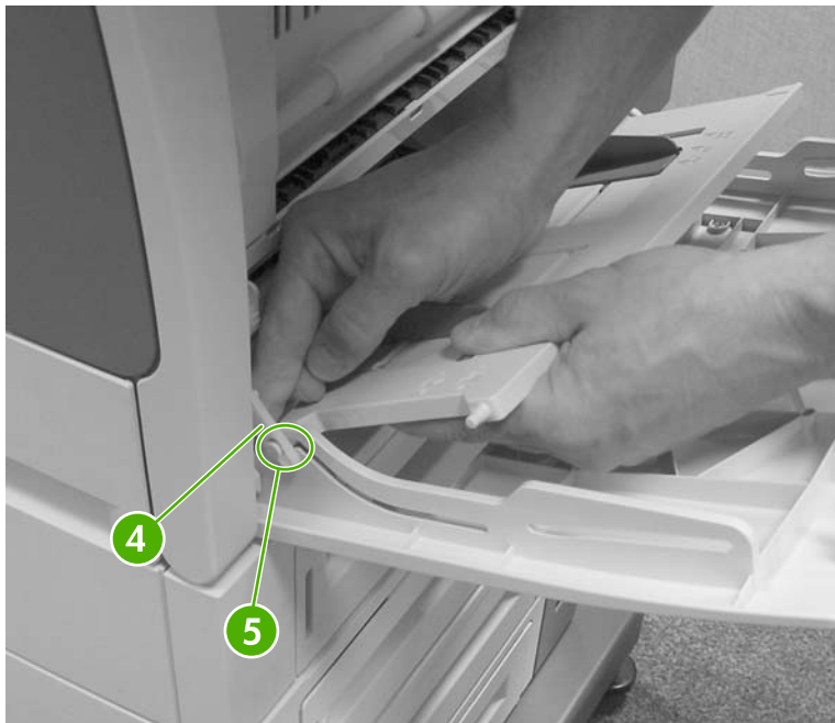
Figure 6-20 Remove the multipurpose tray (4 of 7)
