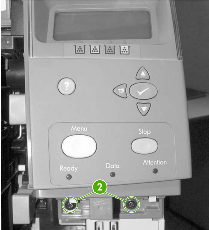
Figure 6-50 Remove the control panel (2 of 3)
