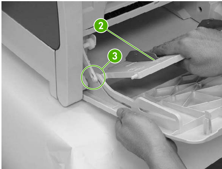
Figure 6-19 Remove the multipurpose tray (3 of 7)
