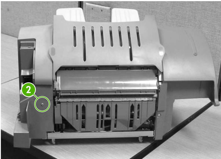
Figure 6-186 Remove the left cover (2 of 2)
