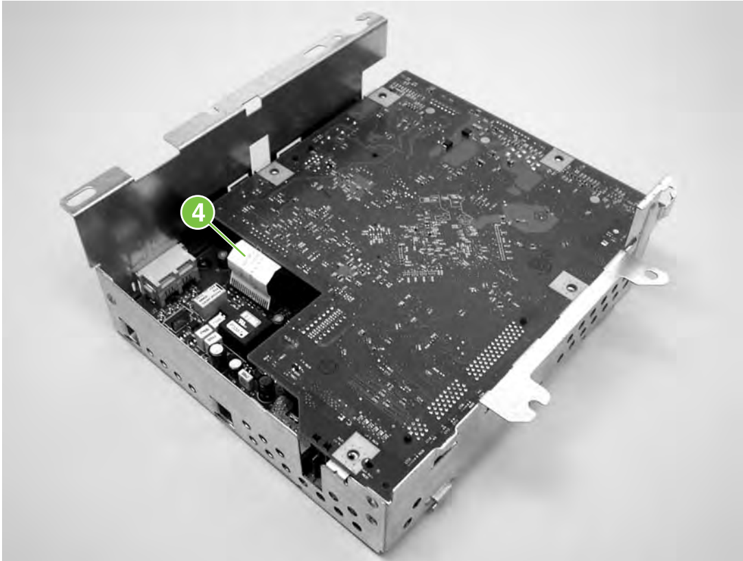
Figure 5-63 Remove the formatter (2 of 2)
