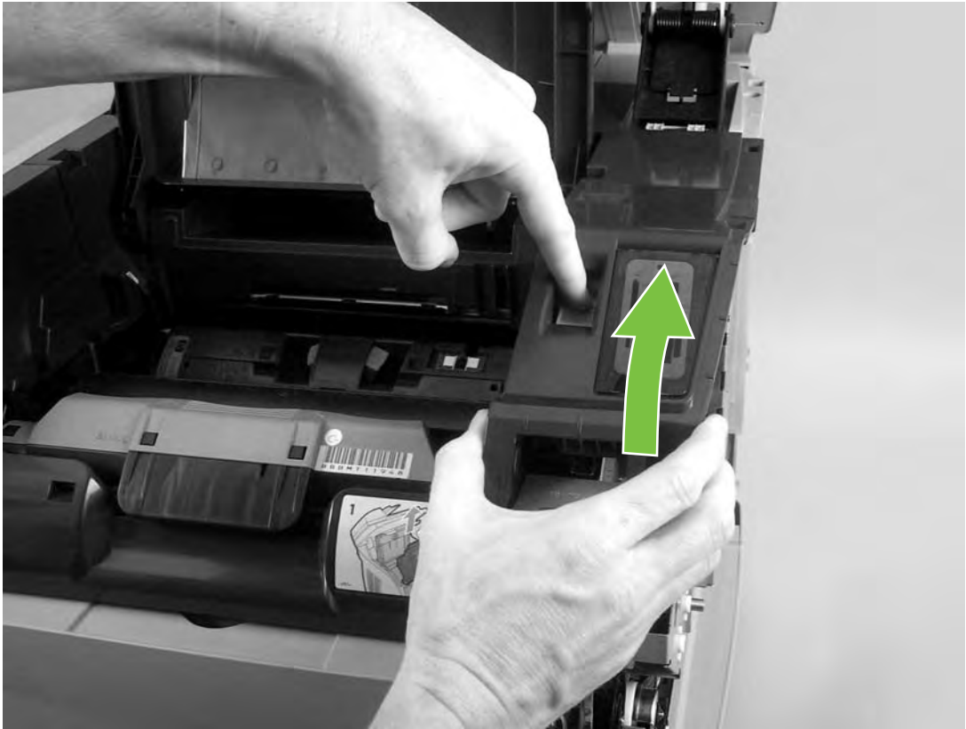
Figure 5-35 Remove the right upper cover (2 of 2)
