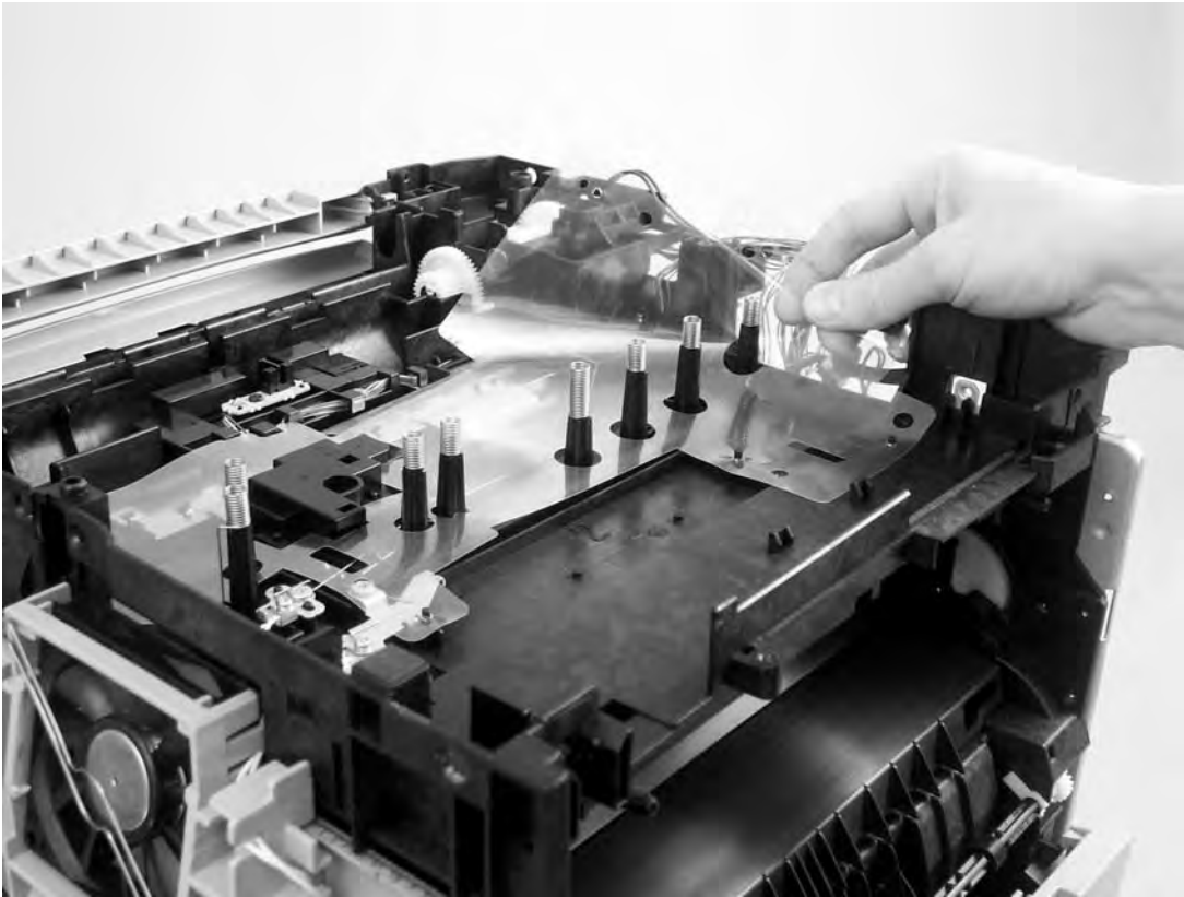
Figure 5-86 Replacing the feed-drive shaft and belts (1 of 8)
