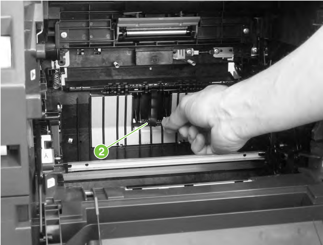
Figure 5-88 Replacing the feed-drive shaft and belts (3 of 8)
