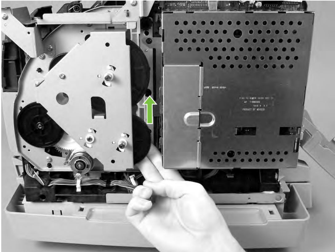
Figure 5-43 Reinstall the link gear
