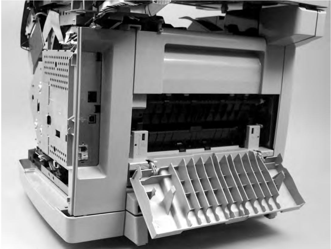
Figure 5-37 Remove the I/O cover (1 of 3)
