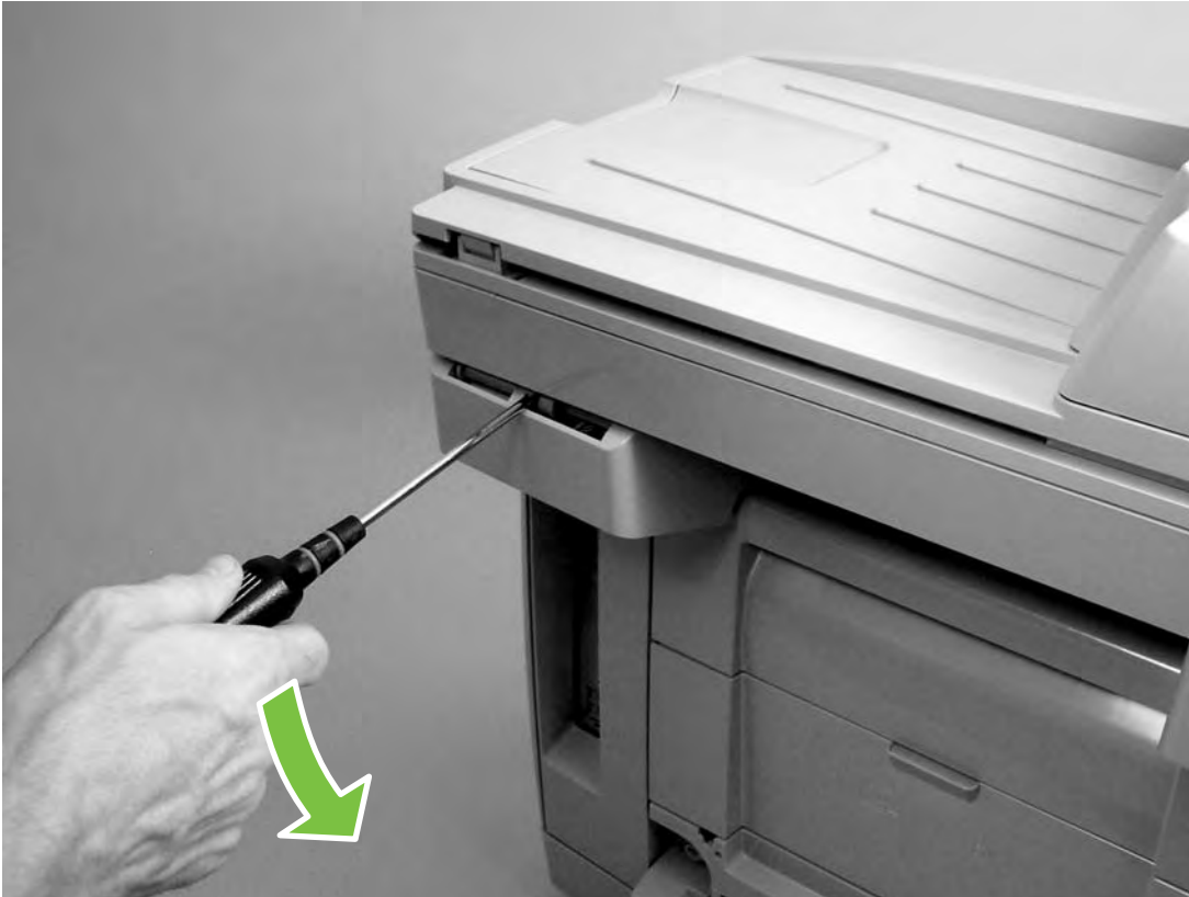
Figure 5-26 Remove the right rear cover (2 of 2)
