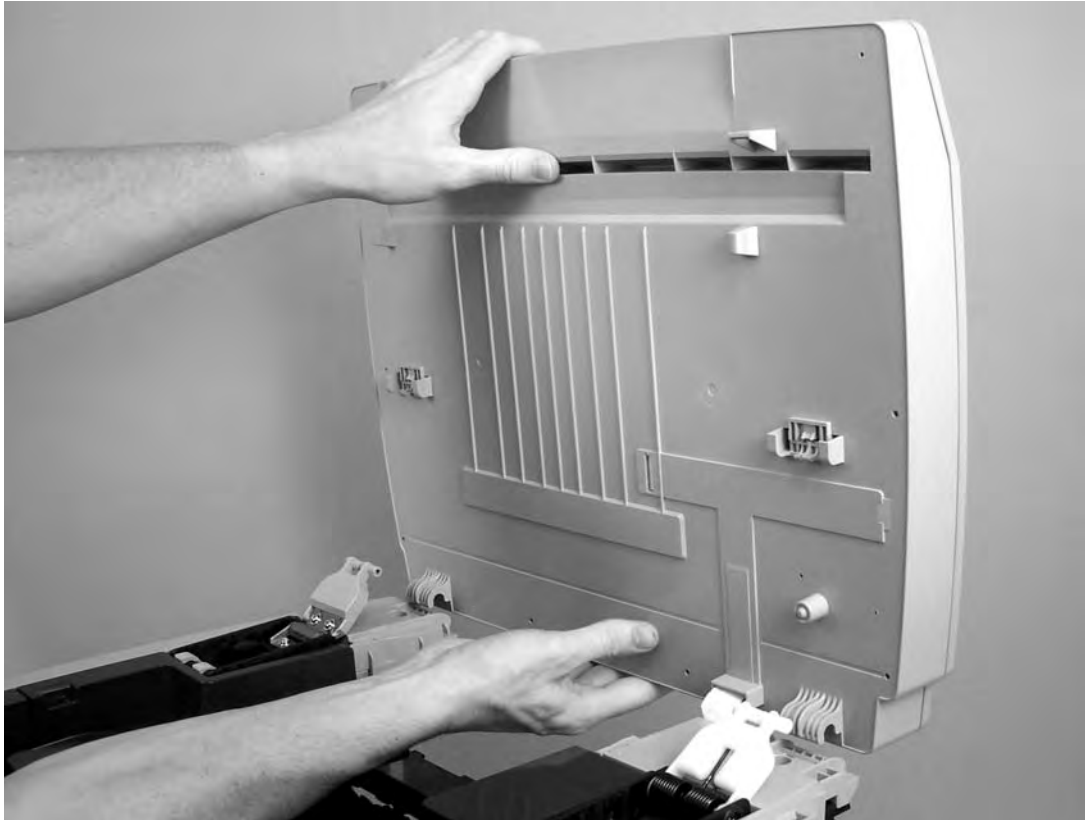
Figure 5-30 Remove the scanning assembly from the device (4 of 4)
