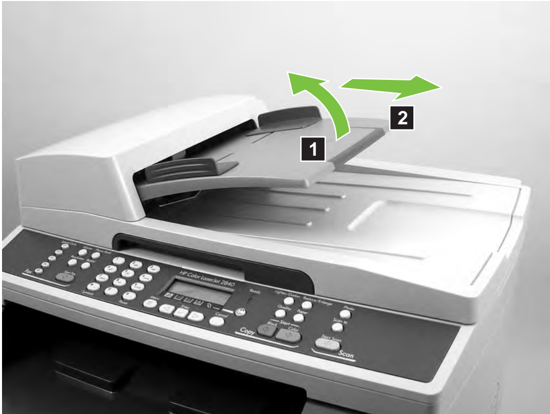
Figure 5-8 Remove the ADF pickup-roller assembly (1 of 5)
