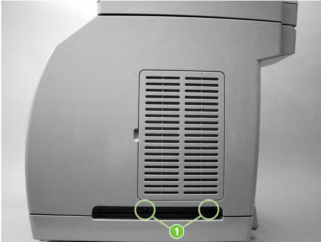
Figure 5-23 Remove the right-side cover (1 of 2)
