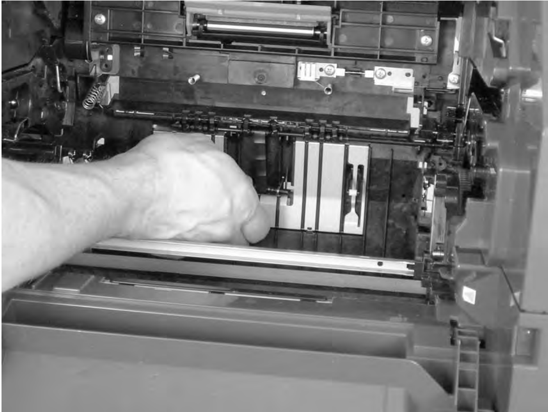
Figure 5-93 Replacing the feed-drive shaft and belts (8 of 8)
