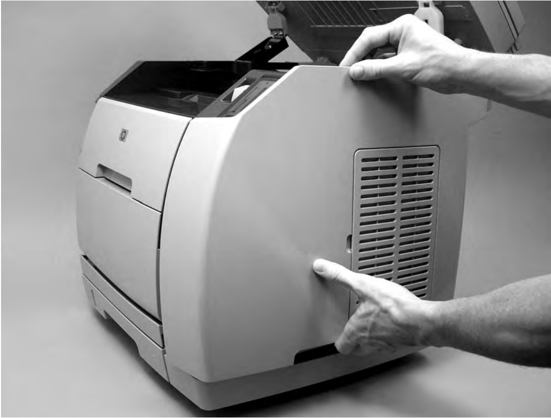
Figure 5-24 Remove the right-side cover (2 of 2)
