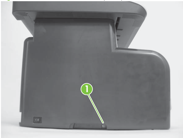
Figure 6-40 Remove the left cover (1 of 4)
