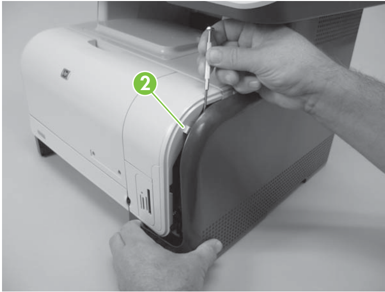
Figure 6-37 Remove the right cover (3 of 5)
