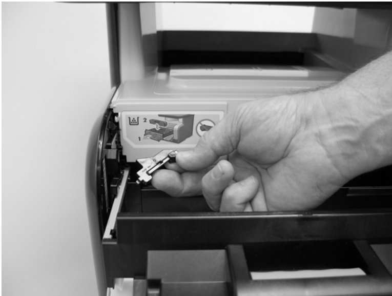
Figure 6-69 Remove the print-cartridge drawer (4 of 5)
