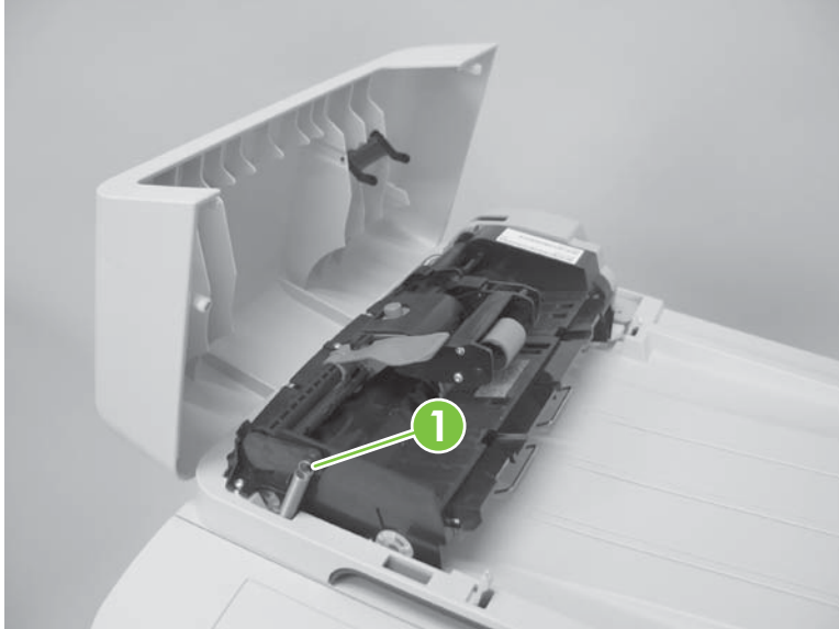
Figure 6-13 Remove the ADF pickup roller assembly (1 of 2)
