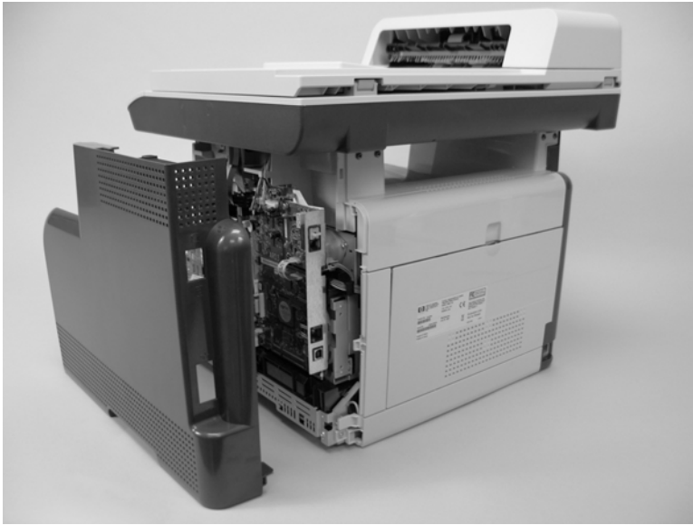
Figure 6-39 Remove the right cover (5 of 5)
