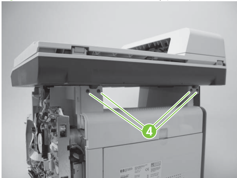
Figure 6-60 Remove the scanner assembly (2 of 4)
