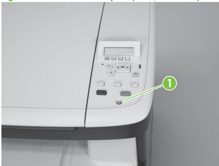
Figure 6-5 Remove the control-panel (1 of 3; base model)
