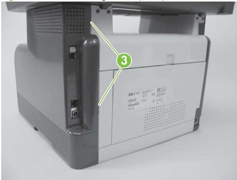
Figure 6-38 Remove the right cover (4 of 5)
