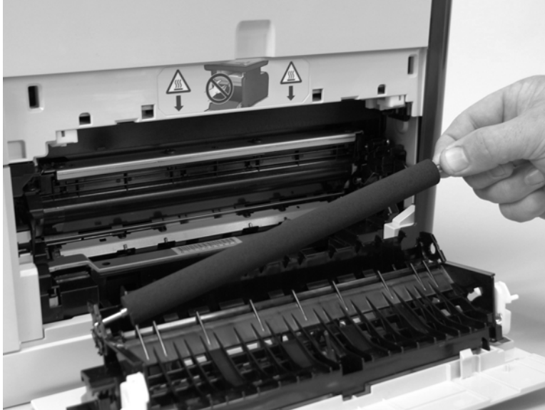
Figure 6-19 Remove the transfer roller (3 of 3)
