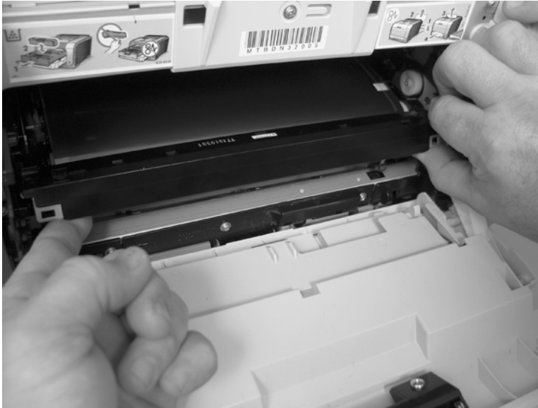
Figure 6-32 Remove the ITB (4 of 6)
