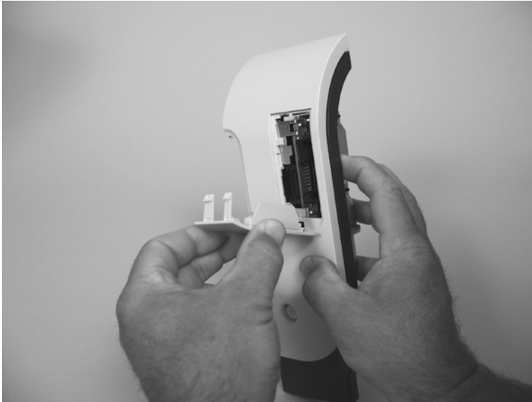
Figure 6-130 Remove the memory-card cover and PCA (6 of 7)
