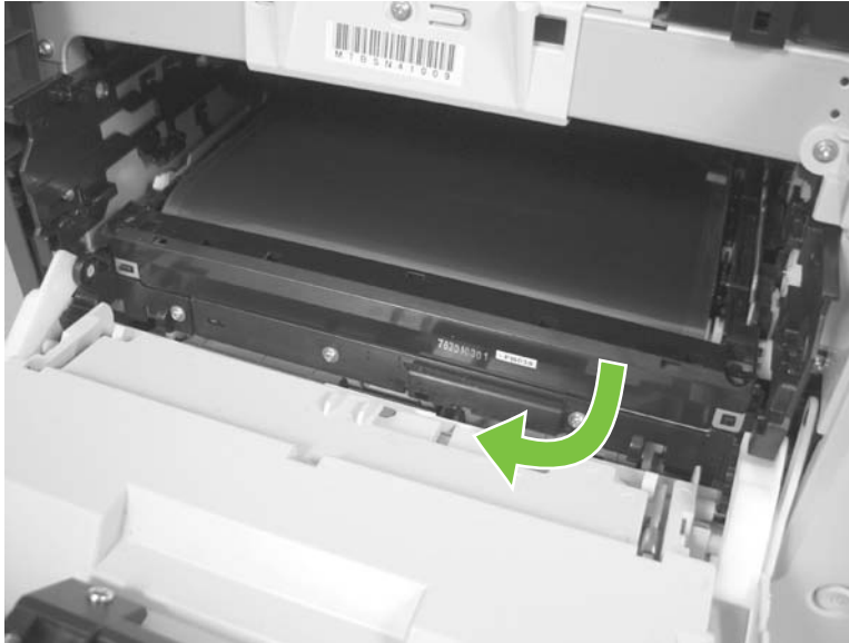
Figure 6-30 Remove the ITB (2 of 6)
