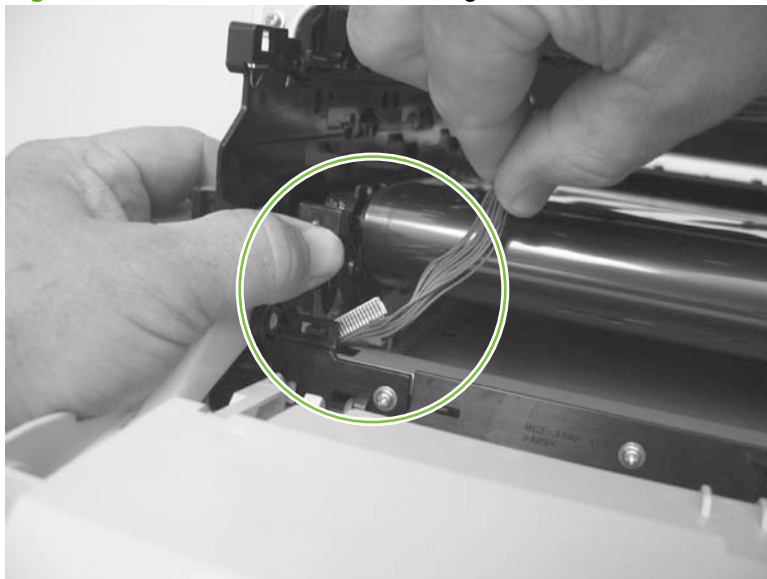
Figure 6-116 Reinstall the color-misregistration sensor assembly PCA (1 of 2)
