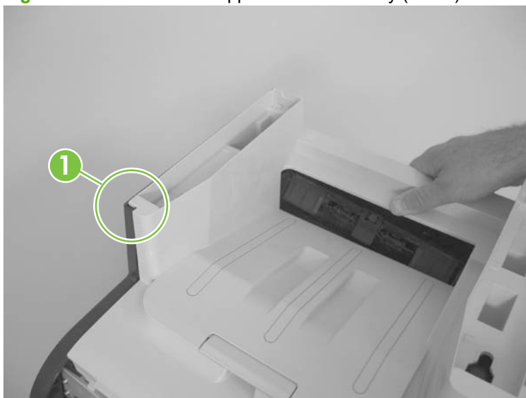
Figure 6-97 Reinstall the upper-cover assembly (1 of 3)
