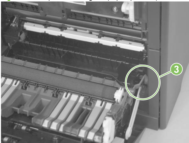
Figure 6-23 Replace the link guide (duplex products)
