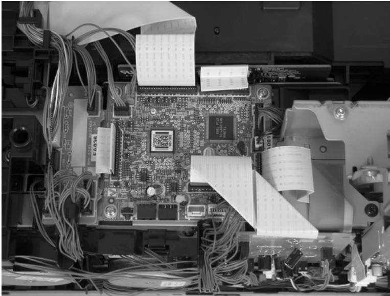
Figure 6-60 Remove the DC controller PCA (1 of 2)
