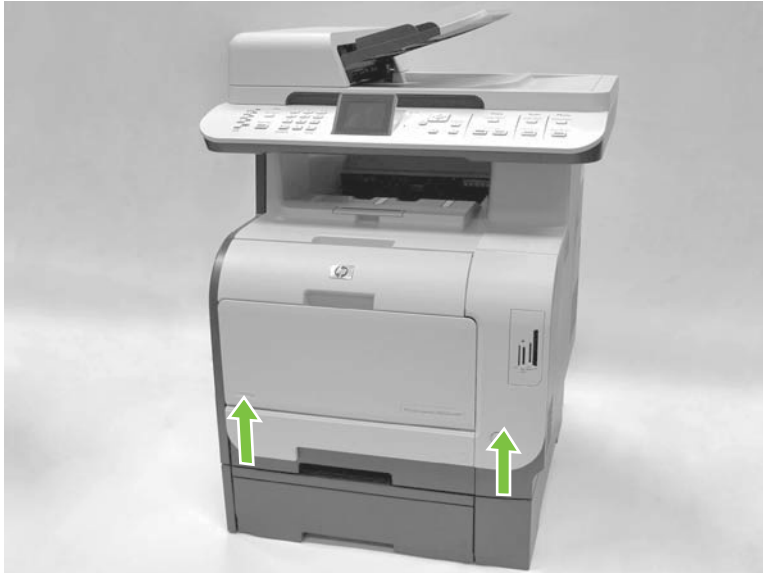
Figure 6-4 Remove the tray cassettes and optional Tray 3 assembly (2 of 2)
