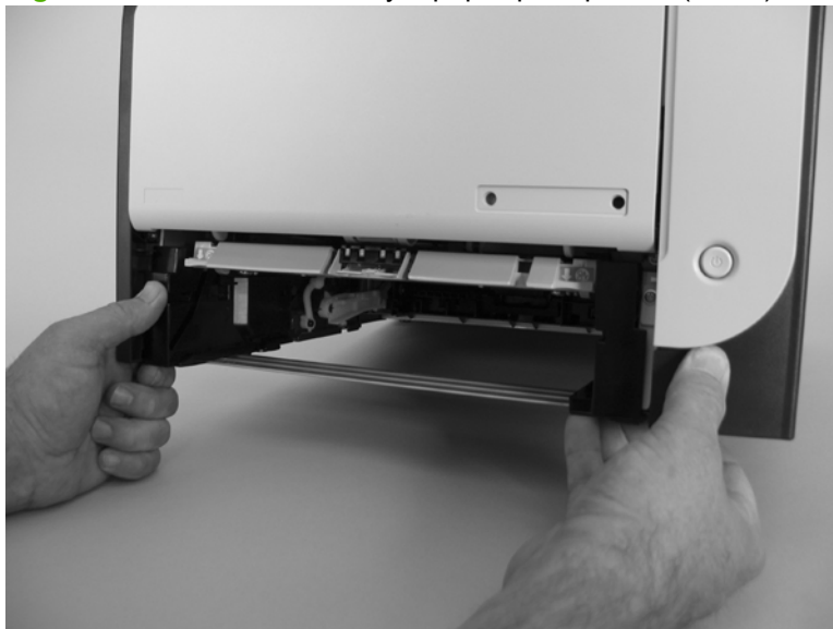
Figure 6-18 Remove the Tray 1 paper-pickup roller (2 of 3)
