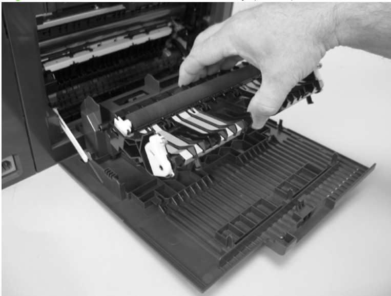
Figure 6-42 Remove the feed assembly (2 of 2)
