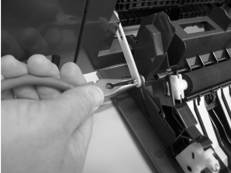
Figure 6-45 Remove the rear door (simplex product) (1 of 4)
