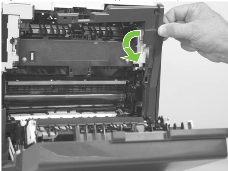
Figure 6-67 Remove the rear-upper cover (2 of 2)
