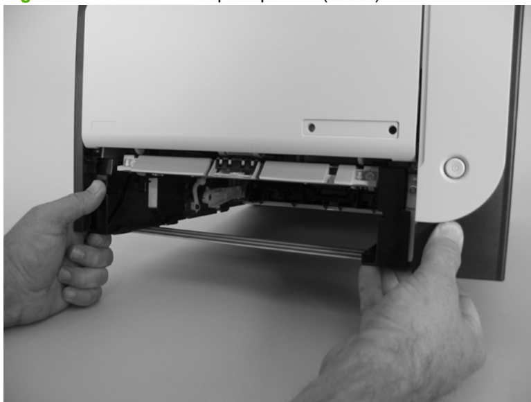
Figure 6-11 Remove the pickup roller (1 of 3)
