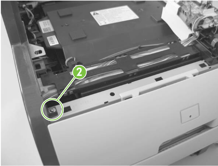
Figure 6-101 Remove the left cover (2 of 4)
