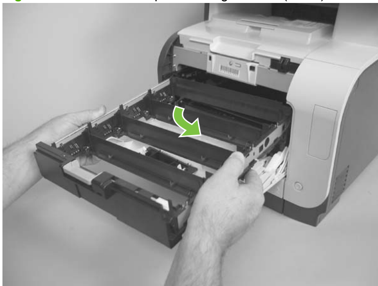
Figure 6-27 Remove the print-cartridge drawer (2 of 3)
