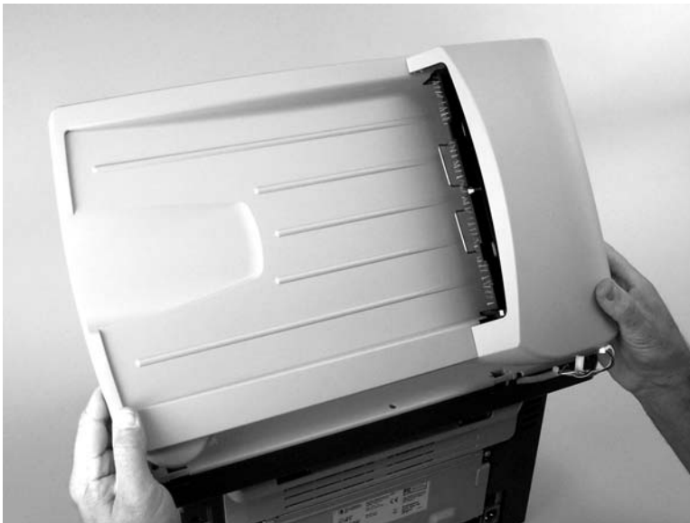
Figure 5-10 Remove the flatbed lid (5 of 5)
