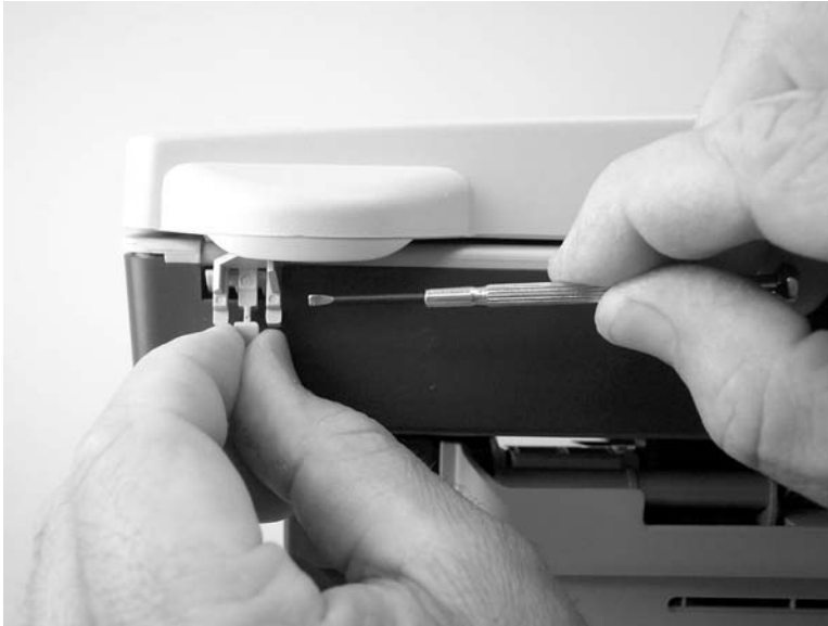
Figure 5-9 Remove the flatbed lid (4 of 5)
