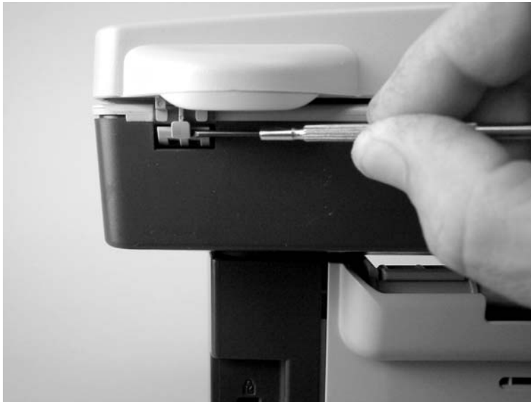
Figure 5-8 Remove the flatbed lid (3 of 5)
