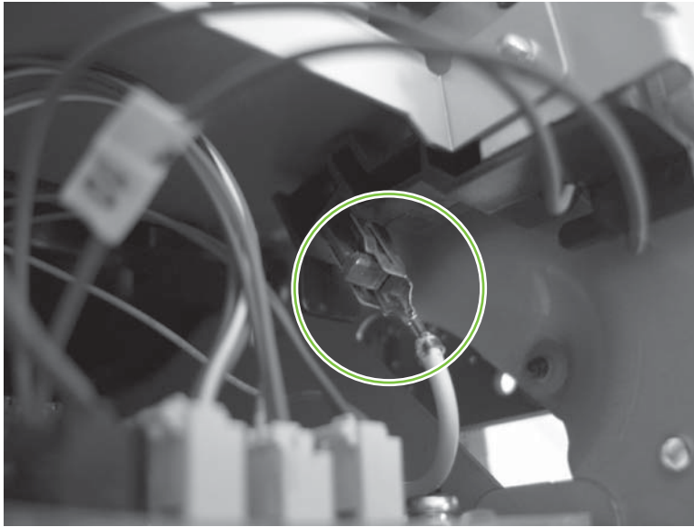
Figure 6-112 Reinstall the fuser (2 of 2)
