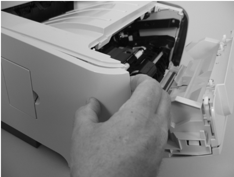
Figure 6-30 Remove the left cover (2 of 4)
