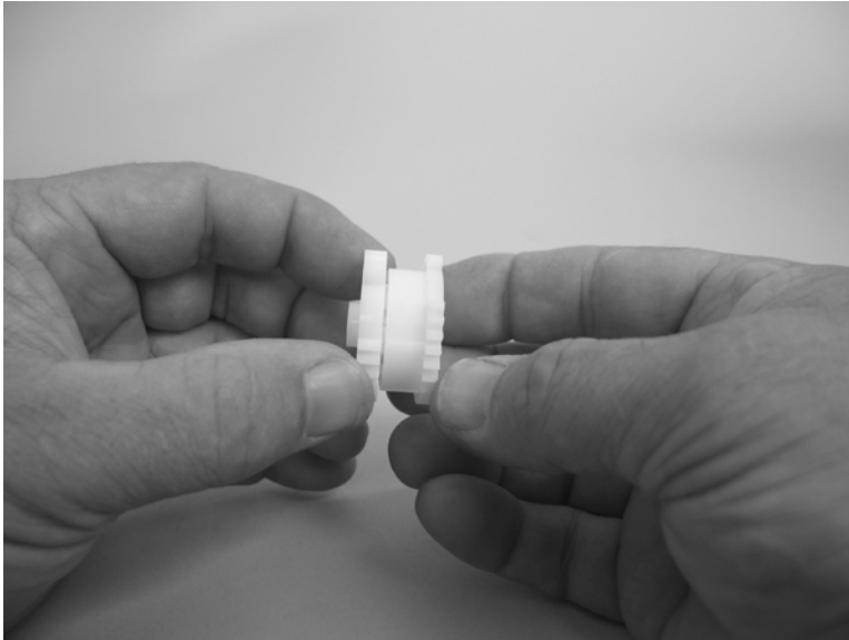
Figure 6-58 Reinstall the paper-pickup-gear assembly (3 of 3)
