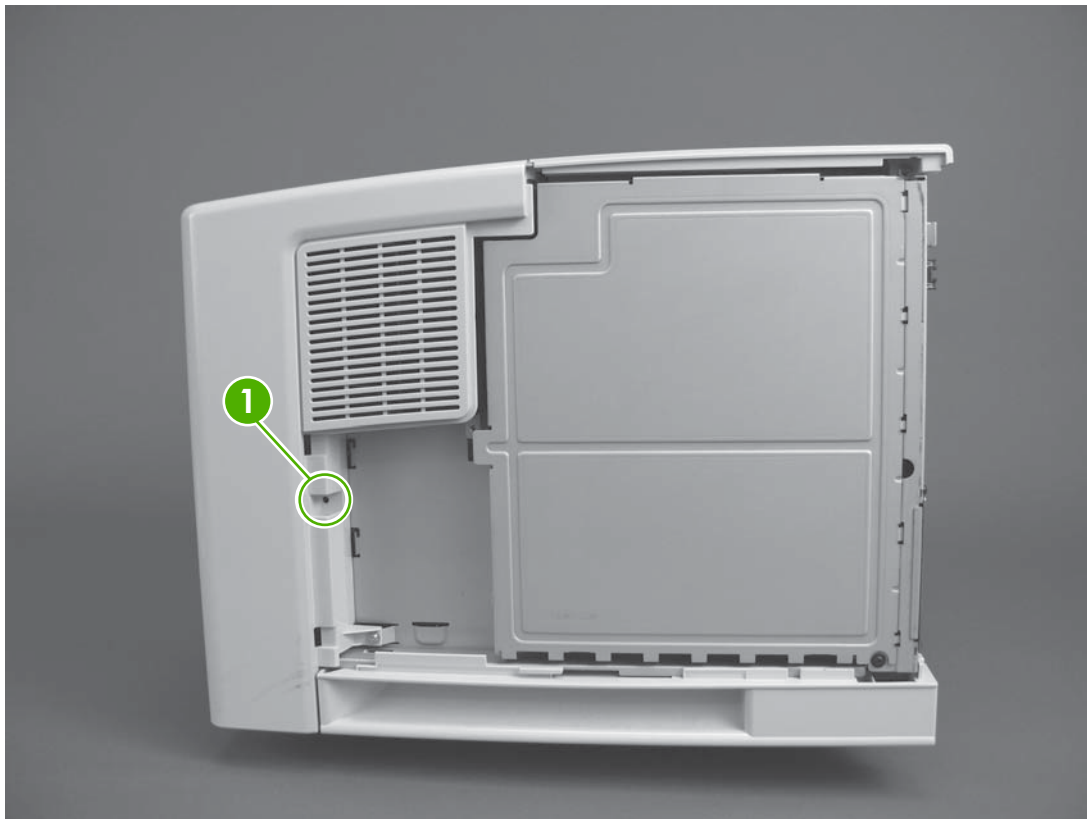
Figure 6-3 Locating the engine-test-page switch
