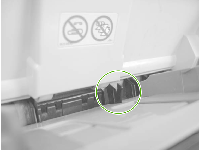
Figure 3-14 Test the Tray 1 (multipurpose tray) media-presence sensor
