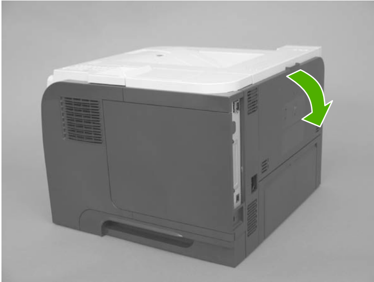
Figure 2-20 Remove the rear-door assembly (1 of 8)
