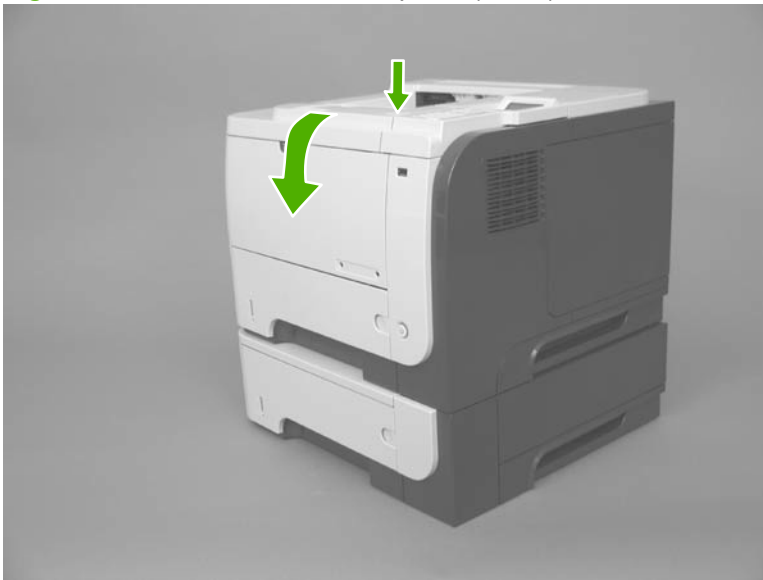
Figure 2-42 Remove the control panel (1 of 4)
