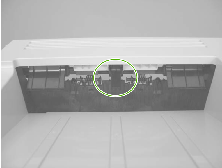
Figure 3-9 Test the face-down media tray media-full sensor
