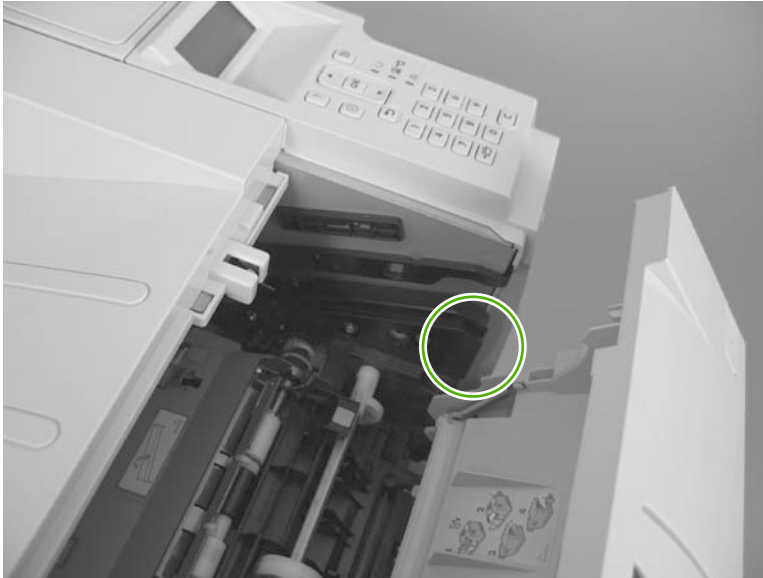
Figure 3-11 Test the cartridge-door open switch
