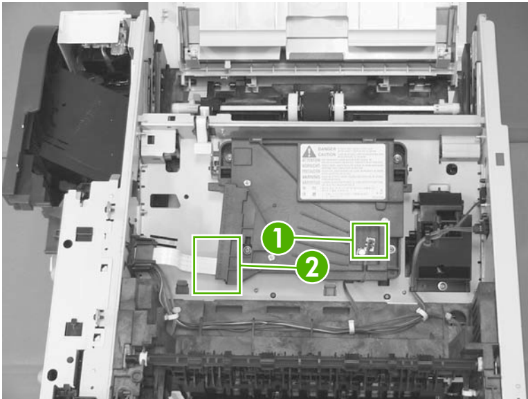
Figure 2-95 Remove the laser/scanner (3 of 5)
