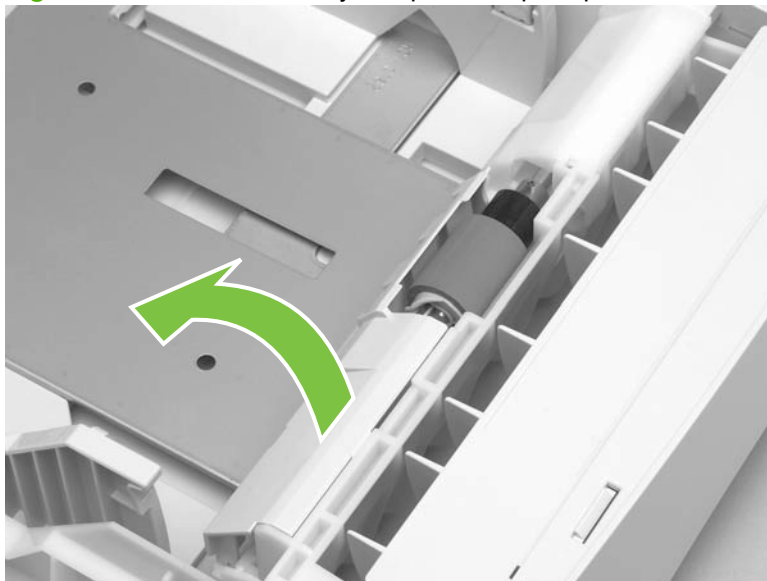
Figure 6-9 Remove the Tray 2 separation, pickup, and feed rollers (1 of 4)
