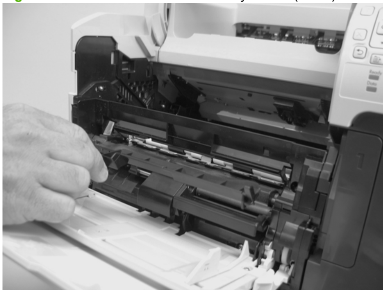
Figure 6-15 Remove the front accessory covers (1 of 2)
