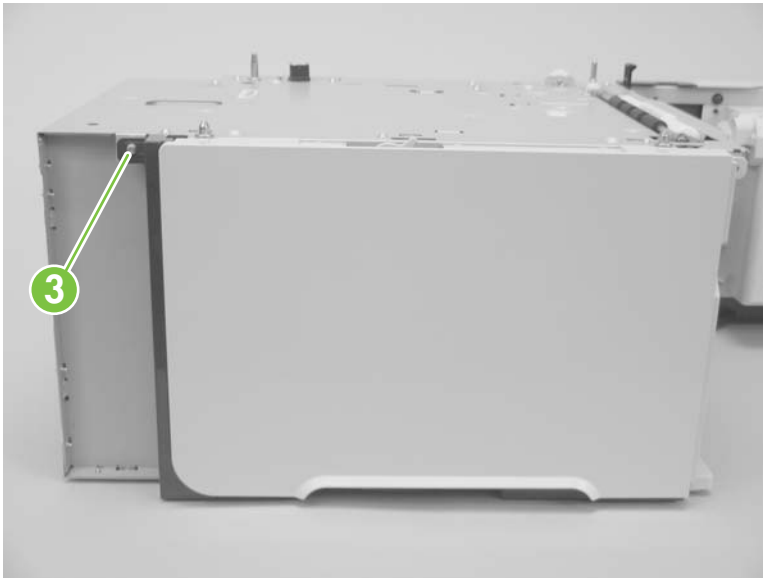
Figure 6-137 Remove the 1,500-sheet feeder left-side cover (4 of 5)
