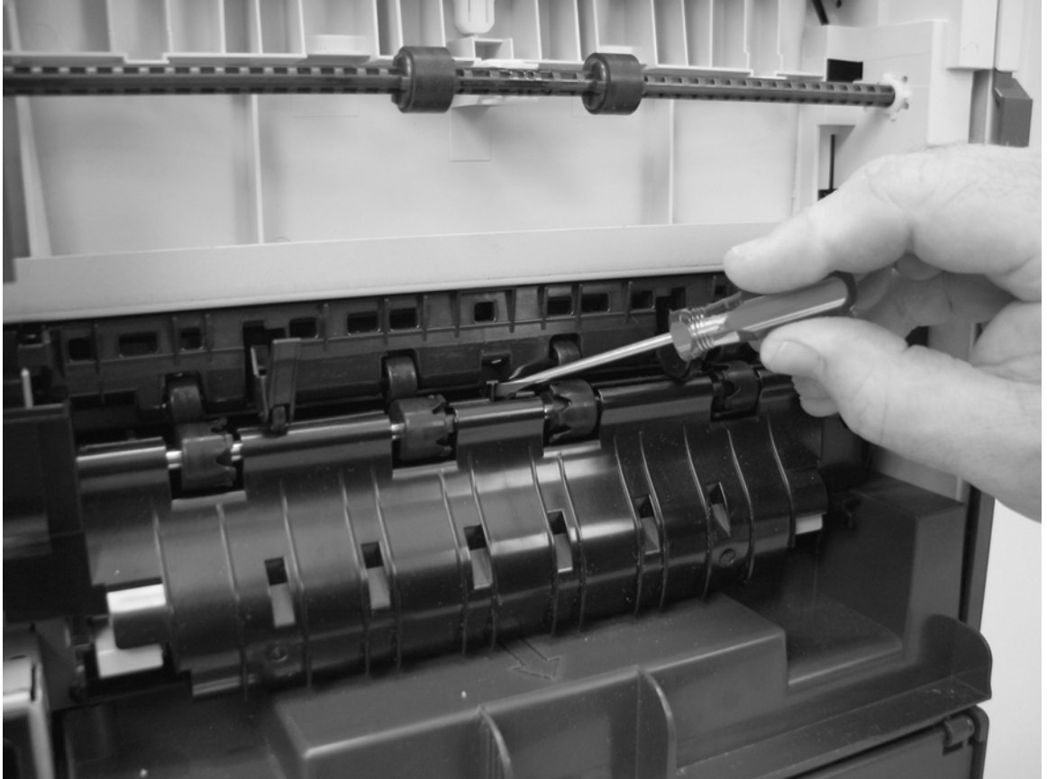
Figure 7-5 Checking the fuser delivery sensor
