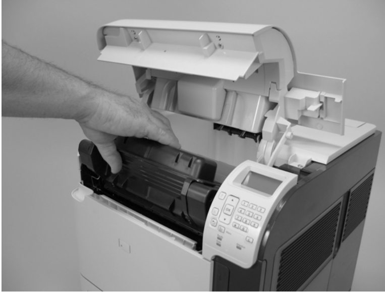
Figure 6-6 Remove the print cartridge (2 of 2)
