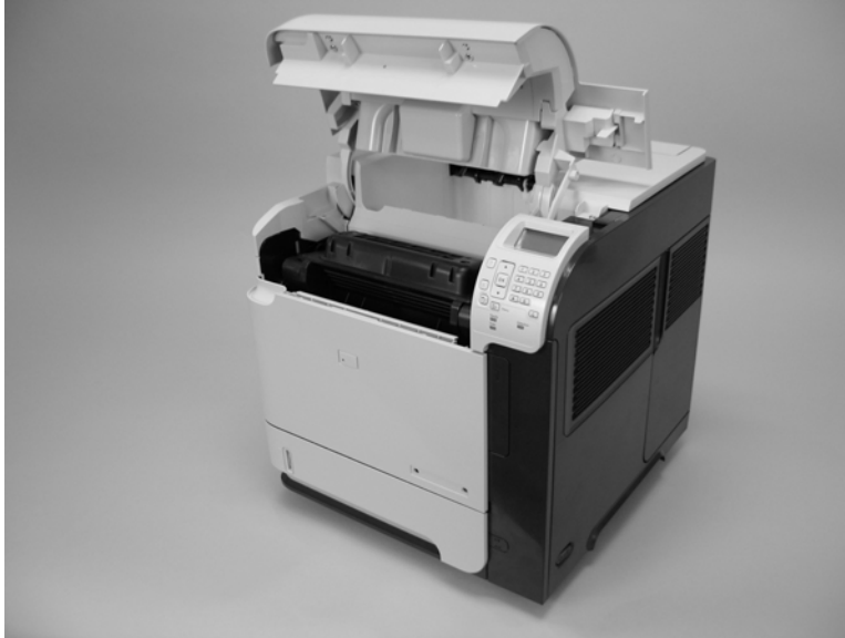
Figure 6-5 Remove the print cartridge (1 of 2)
