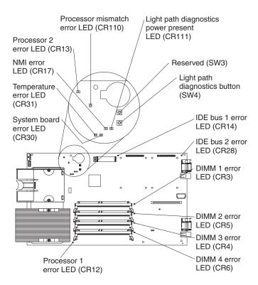
Figure 5. System board: light path diagnostics
