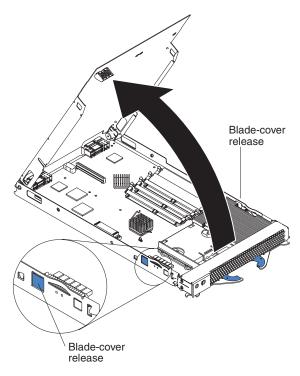
Figure 14. Opening the blade server cover
