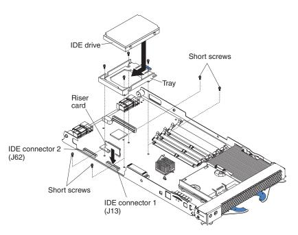
Figure 18. Installing an IDE drive
