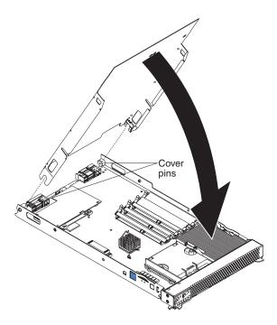
Figure 15. Closing the blade server cover
