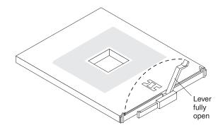
Figure 22. Microprocessor locking lever in the fully open position
