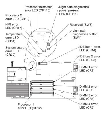
Figure 31. System board LED locations
