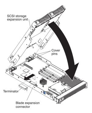
Figure 25. SCSI storage expansion unit installation
