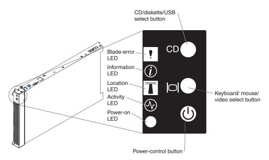
Figure 4. Controls and LEDs
