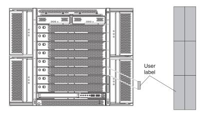
Figure 3. Label placement, Blade Center T unit
