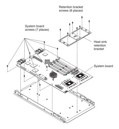
6. Remove the eight screws that secure the heat sink retention bracket to the system board, and put the screws and the module in a safe place.
