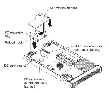
Figure 24. Installing an I/O expansion card
