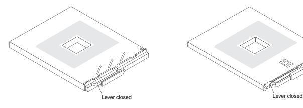
Figure 27. Microprocessor locking lever in the closed position
