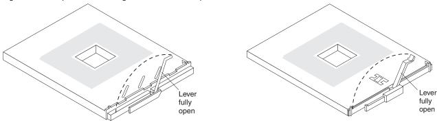
Figure 28. Microprocessor locking lever in the fully open position
