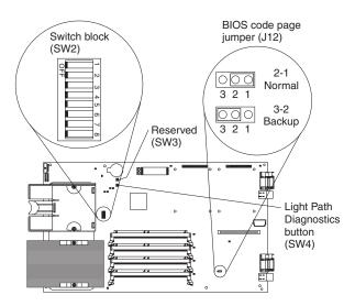
Figure 30. System board switches and jumpers
