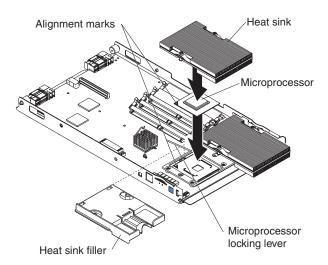
Figure 20. Installing a second microprocessor
