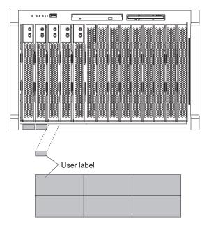
Figure 2. Label placement, Blade Center unit
