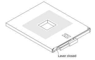
Figure 21. Microprocessor locking lever in the closed position
