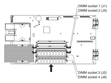
Figure 19. DIMM socket locations
