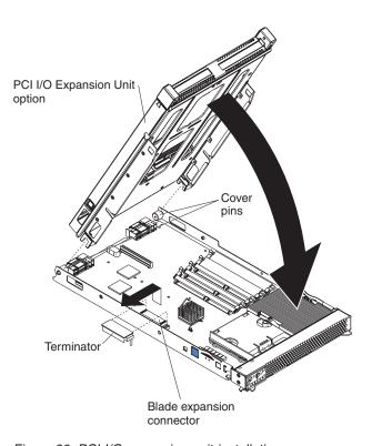
Figure 26. PCI I/O expansion unit installation
