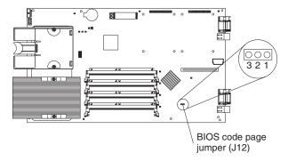
Figure 6. System board: BIOS code page jumper
