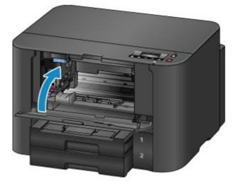
After ink tank replacement, the printer starts mixing the ink automatically. Wait until this noise stops. (Mixing takes 1–2 minutes.)
