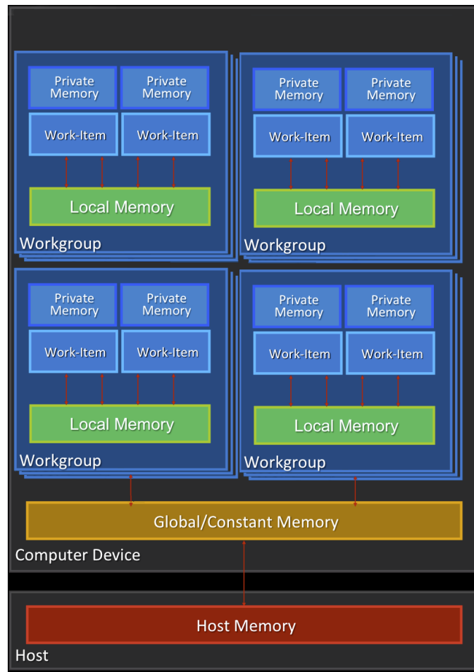
Figure 5 OpenCL Memory Hierarchy
