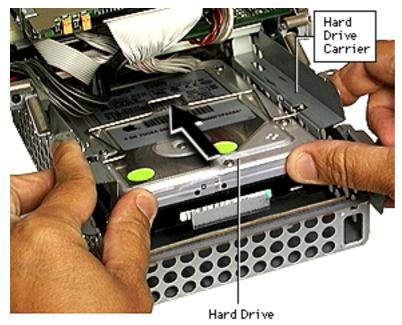
2. Holding on to the hard drive carrier, push the carrier back to free the carrier from the chassis.
