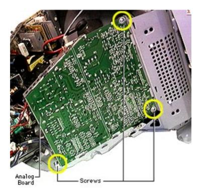
4. Remove the three silver screws on the analog board.
