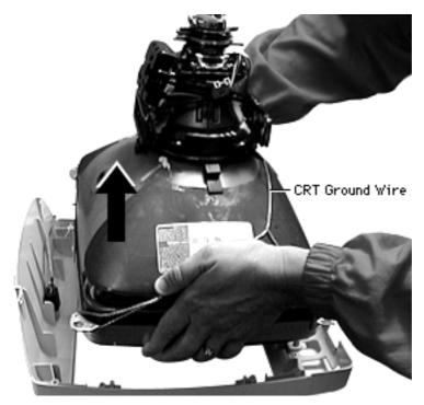
3. Lift the CRT off the front inner bezel.
