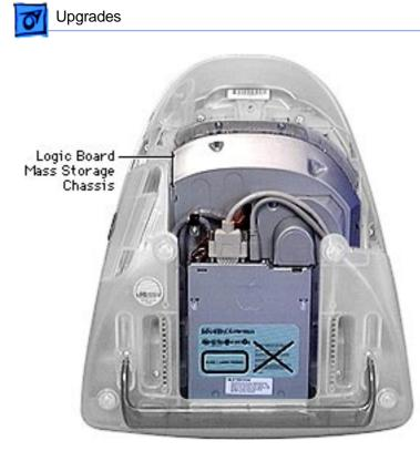
Remove the two screws at the top of the logic board/mass storage chassis and disconnect the cables and screw clamp.
