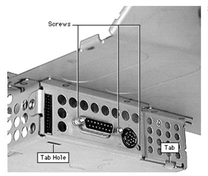
2. Remove the two thumbscrews (with a nut driver) and the one phillips screw from the outside of the board.
