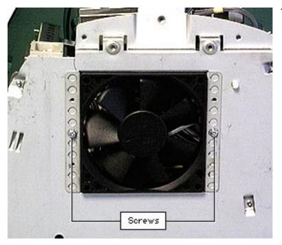
1. Remove the two screws from the fan bracket.
