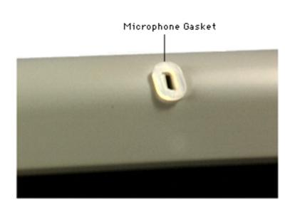
Place the gasket around the microphone opening in a vertical orientation. Ensure that the microphone opening is not obstructed by the gasket.
