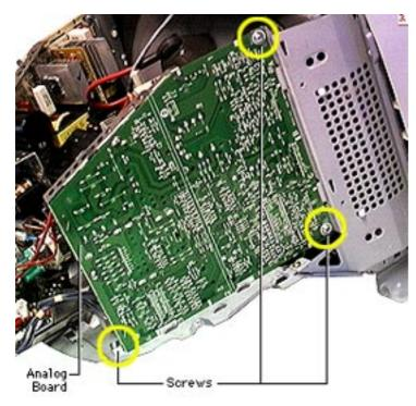
4. Remove the three screws on the analog board.
