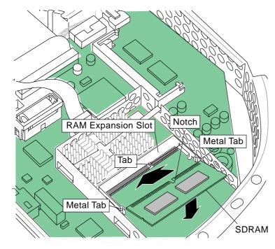
Line up the notch in the SDRAM DIMM with the small plastic tab in the SDRAM slot. Push in on the card and then down until the two metal snaps click into place.L
