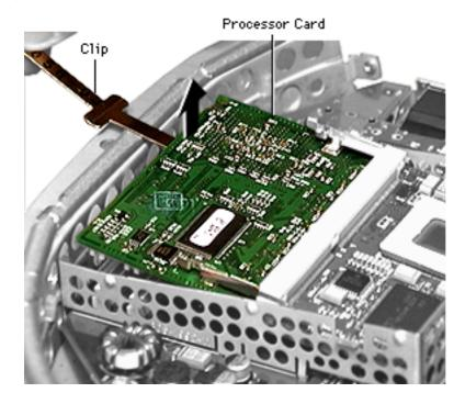
Pry the processor card from the logic board connectors. This can be done with a spring hook removal tool or carefully with the heatsink clip as shown in the graphic.
