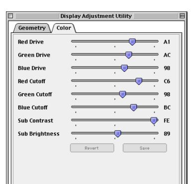
5. Adjust the Sub Contrast slider to increase the screen brightness until the luminance measures correctly.
