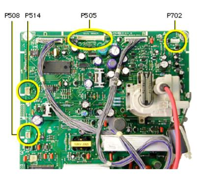
Disconnect P702, P505, P514, and P508 and a 4-pin multi-color CRT cable (not shown).
