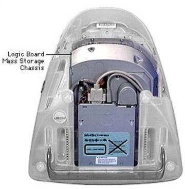
2. Remove the two screws at the top of the logic board/mass storage chassis and disconnect the cables and screw clamp.
