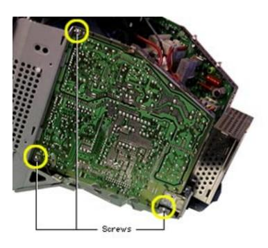
Remove the three silver screws on the power supply board.
