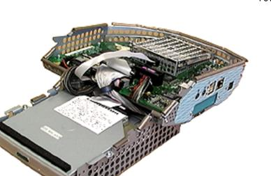
10. Place the logic board/ mass storage chassis on an ESD mat.
