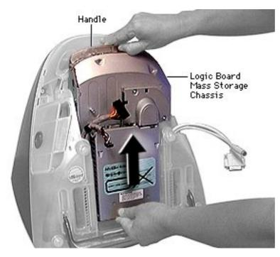
Using the handle, pull up on the chassis and slide the logic board/mass storage chassis out of the unit.
