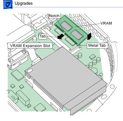
11. Line up the notch in the SGRAM DIMM expansion card with the small plastic tab in the VRAM expansion slot. Push in on the VRAM card, and then down, until the two metal snaps click into place.
