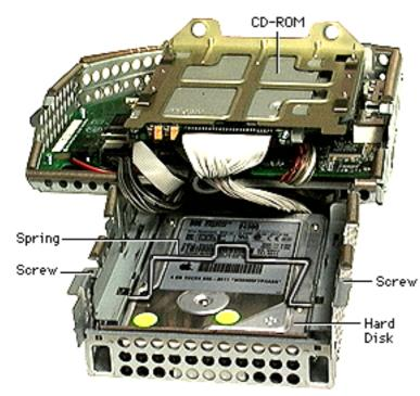
1. Remove the two screws securing the hard drive carrier to the chassis.
