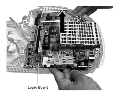
5. Holding the logic board by its edges, gently lift the logic board to disconnect it from the power filter board located underneath.
