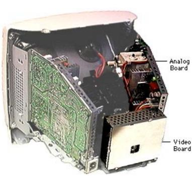
The following procedure is for the 661-2166 Ver. 2 analog/video board.
