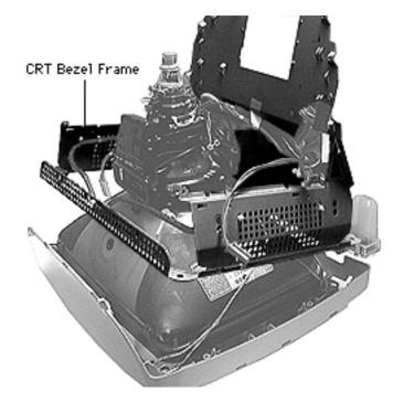
2. Lift the CRT bezel frame off the CRT.
