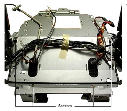
Remove the four brasscolored screws to separate the top frame from the bottom frame.R
