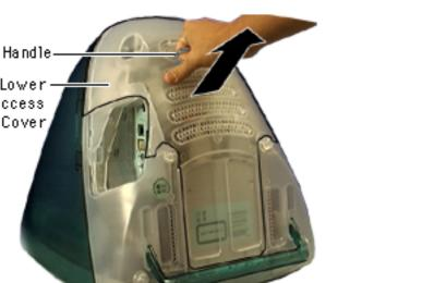
2. Using the handle, quickly jerk the lower access cover up and towards you.
