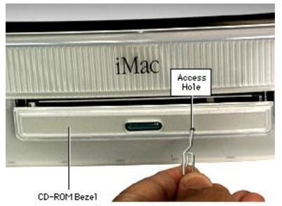
Open the CD-ROM drive drawer by gently pushing a paper clip into the access hole.
