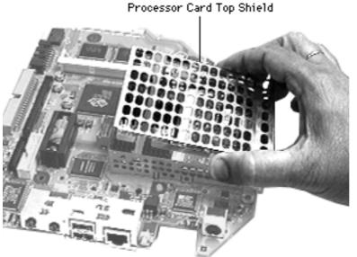
1. Remove the top shield from the processor card.
