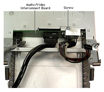
Remove the silver screw from the EMI shield on the audio/video interconnect board.
