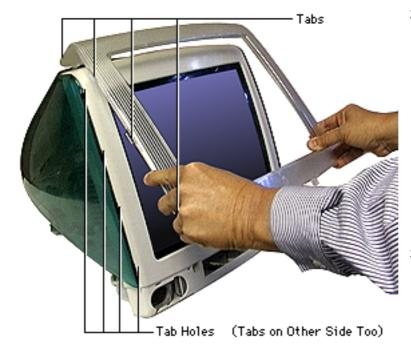
2. With the CRT facing you, use a plastic tool to push in the tabs on the left side and then on the right side to release the tabs from the bezel holes. Start pushing the tabs in from the bottom left corner and work your way to the top.
