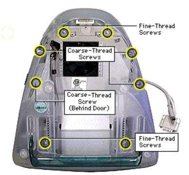
1. Remove the eight screws on the bottom housing.
