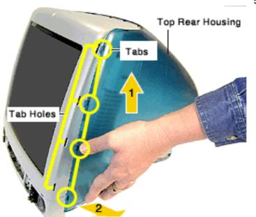
5. **Note:** There are tab holes on both sides of the front inner bezel
