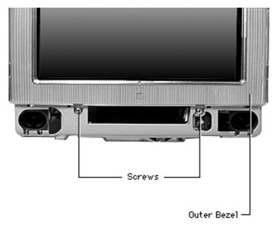
3. Replace the two front bezel screws.
