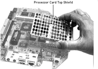
5. Remove the processor card top shield.
