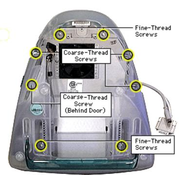
1. Remove the the eight bottom housing screws.
