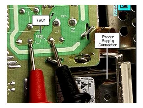
**Testing the Power Supply Board Fuse**
