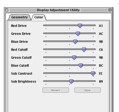
Adjust the red, green, and blue cutoff controls until the second bar (from the left) is barely visible.
