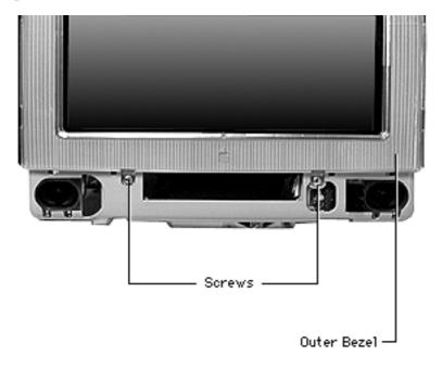
1. Remove two screws on the front outer bezel.
