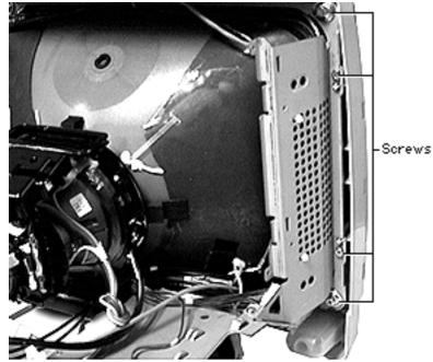
Remove the eight screws attaching the CRT frame to the inner plastic bezel. There are four screws on each side.
