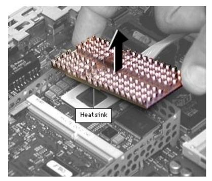
3. Lift the heatsink off the processor card.
