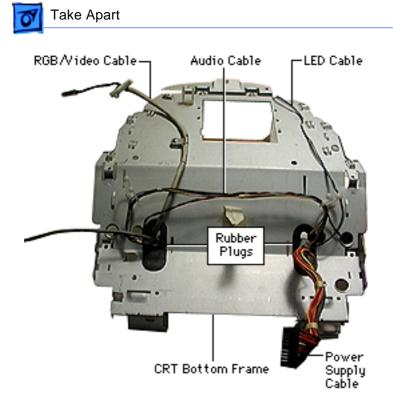
4. The remaining frame is the CRT bottom frame. It ships without the cables and rubber plugs.
