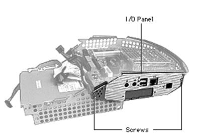
1. Remove the two screws that secure the I/O panel to the chassis.
