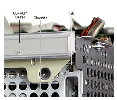
2. Ensure the metal tabs on the CD carrier feed into the tab holes on the chassis to secure the CD-ROM drive in place.
