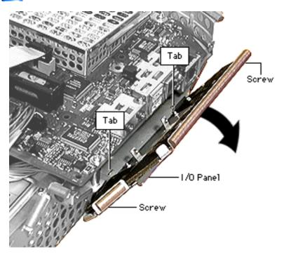
Tilt the I/O panel outward and unhook the I/O panel tabs from the chassis.
