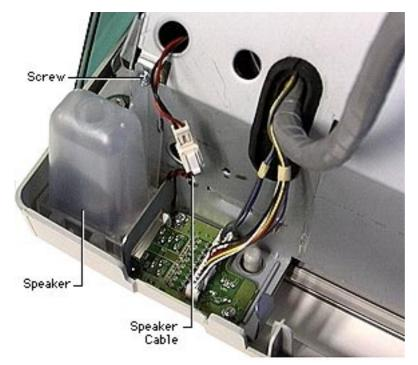
3. Lift speaker up and out of the chassis frame.
