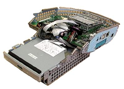
4. Place the logic board/mass storage unit on an ESD mat.
