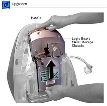
Using the handle, pull the main logic board/ mass storage chassis from the unit.
