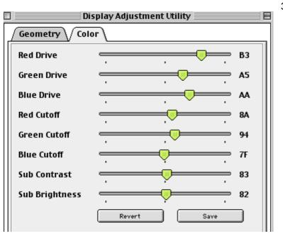
Select the Color tab window and move the Sub Contrast and Sub Brightness controls to midrange.
