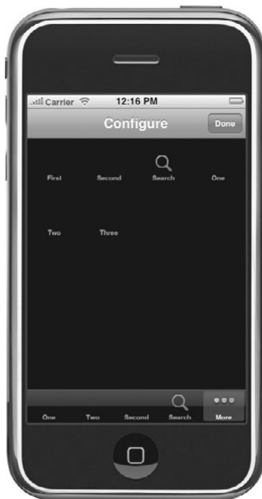
Figure 8-12 Clicking Edit displays a view for configuring the tab bar's tabs.
