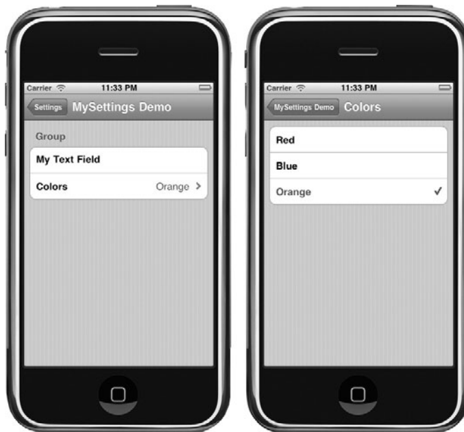
Figure 14-9 Settings reflecting the new setting
