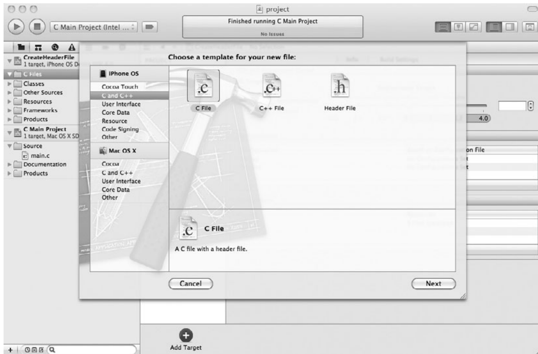
Figure 2-2 Adding a C file to the project using the New File dialog
