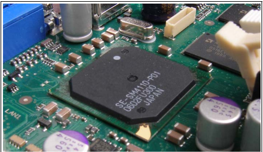
Figure 1: iRMC S2 on the system board of a PRIMERGY server
