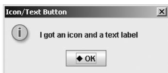
Figure 9-11. Using JOptionPane with a JButton containing a text label and an icon
