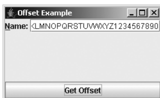
Figure 15-4. The scrollOffset property reflects how far to the left the field's contents have scrolled; here, it is not at zero, so the beginning contents (A–J) have scrolled off to the left.
