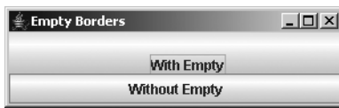
Figure 7-3. EmptyBorder sample, with insets of 20 for top and left, 0 for right and bottom
