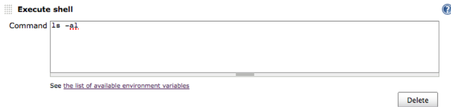
Figure 5.28. Configuring an Execute Shell step
