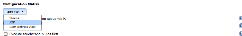
Figure 10.20. Adding an axis to a multiconfiguration build
