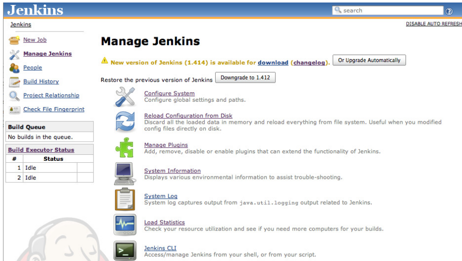
Figure 3.10. Upgrading Jenkins from the web interface
