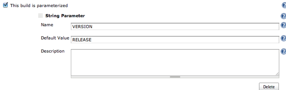
Figure 10.2. Adding a parameter to the build job
