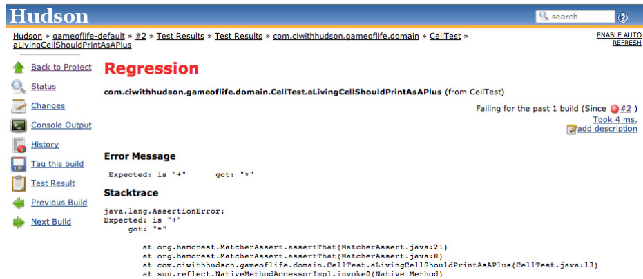
Figure 2.23. Details about a failed test
