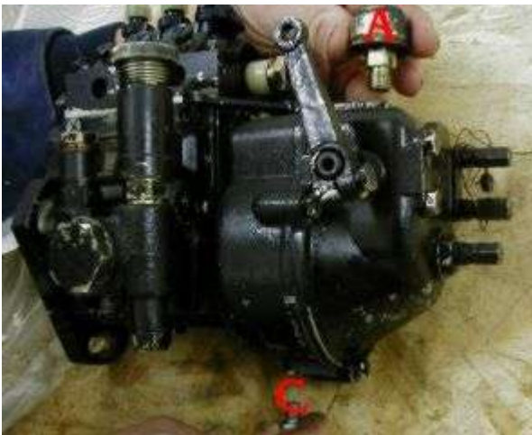
Figure 29. Fuel Injector Oil filler (A) & Drain (C)
