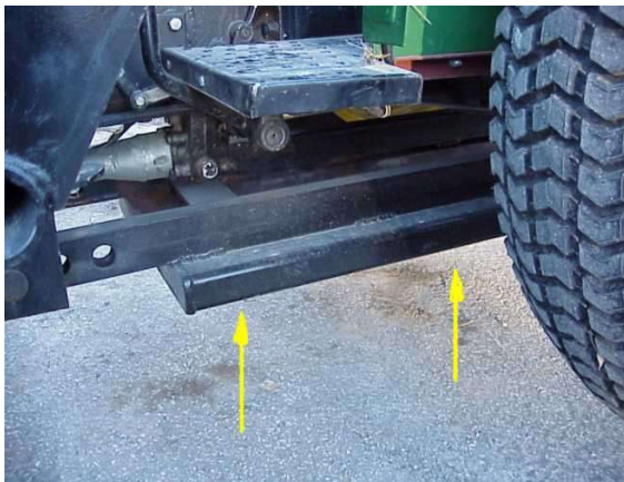
Figure 40. Hoe Frame showing heavy reinforcement
