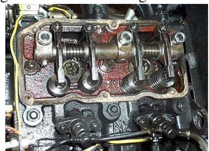
Figure 21. Close-up of JM-204 TY290 engine head
