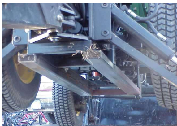
Figure 43. Hoe frame reinforcement after view
