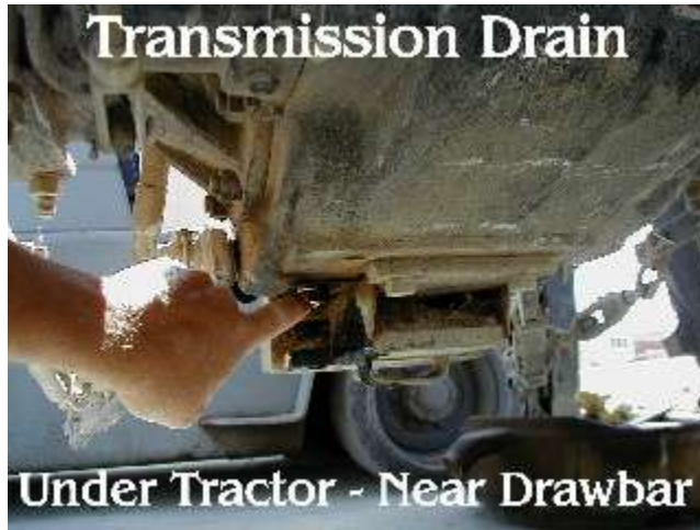
Figure 33. Transmission Oil Drain
