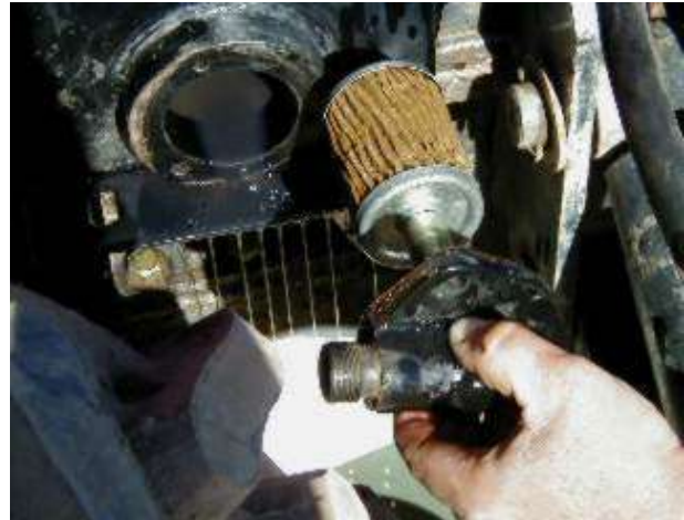
Figure 27. Hoe Hydraulic Oil Filter
