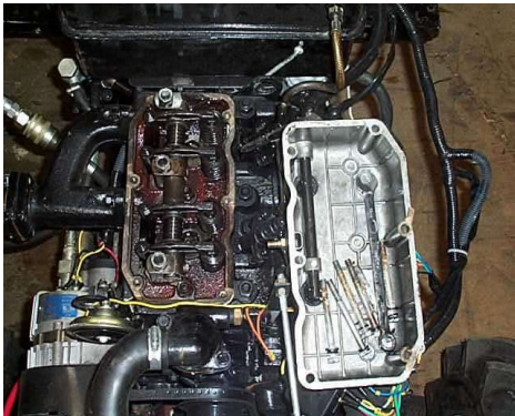
Figure 20. JM204 TY29 Engine with valve cover removed
