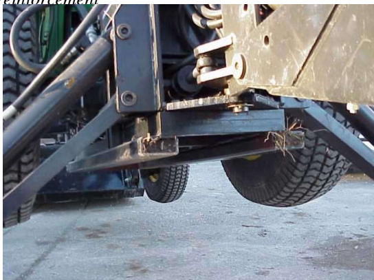
Figure 42. Hoe frame reinforcement fwd view
