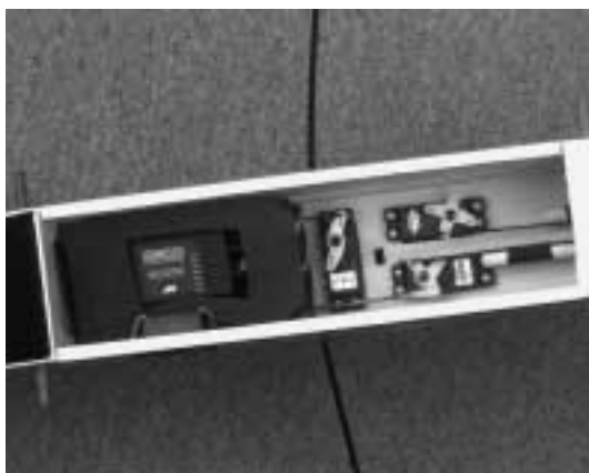
Fuselage Servo, Receiver, Battery Installation
