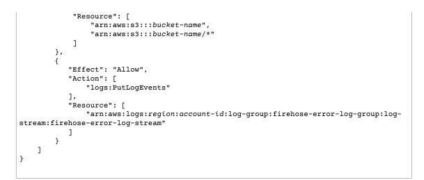
Replace *bucket-name* with a unique bucket name where the logs will be stored. Replace *region* with the AWS Region where the CloudWatch Logs log group and log stream will be created for logging any errors that occur during streaming the data to Amazon S3 via Kinesis Data Firehose. Replace *account-id* with the 12-digit account ID for the account where the log group and log stream will be created.
