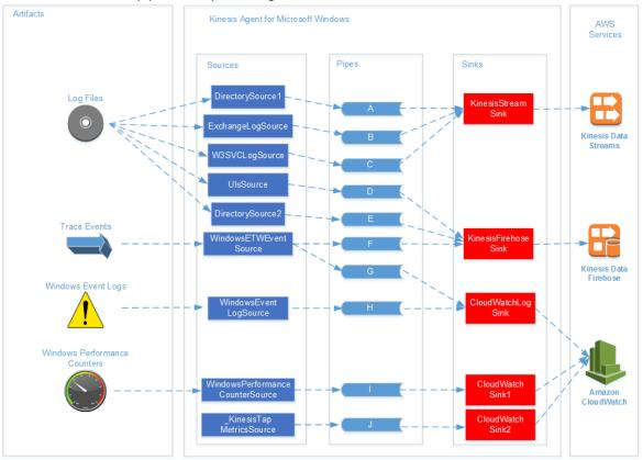
This diagram of a data pipeline illustrates the following components and processes:
