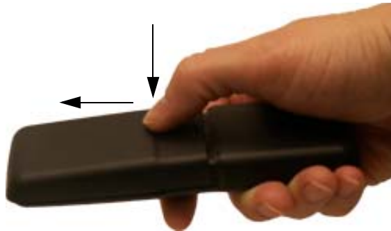
Figure 25 Remove Back Cover from Handset
