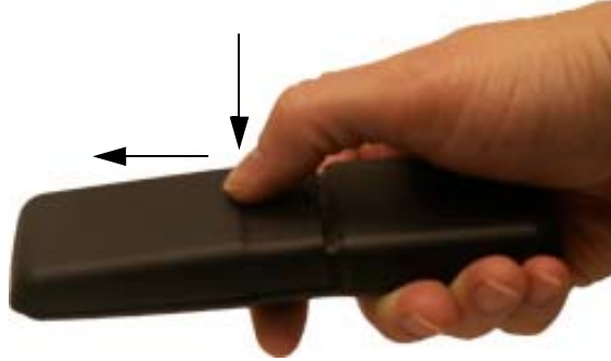
Figure 33 Remove Back Cover from Handset
