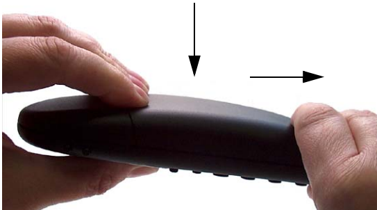
Figure 31 Remove Back Cover from Handset
