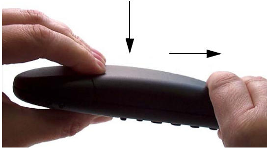
Figure 23 Remove Back Cover from Handset
