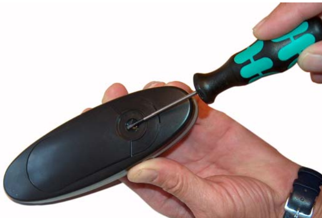
Figure 32 Remove Back Cover from Handset with Screw Fastener
