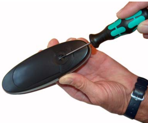
Figure 24 Remove Back Cover from Handset with Screw Fastener
