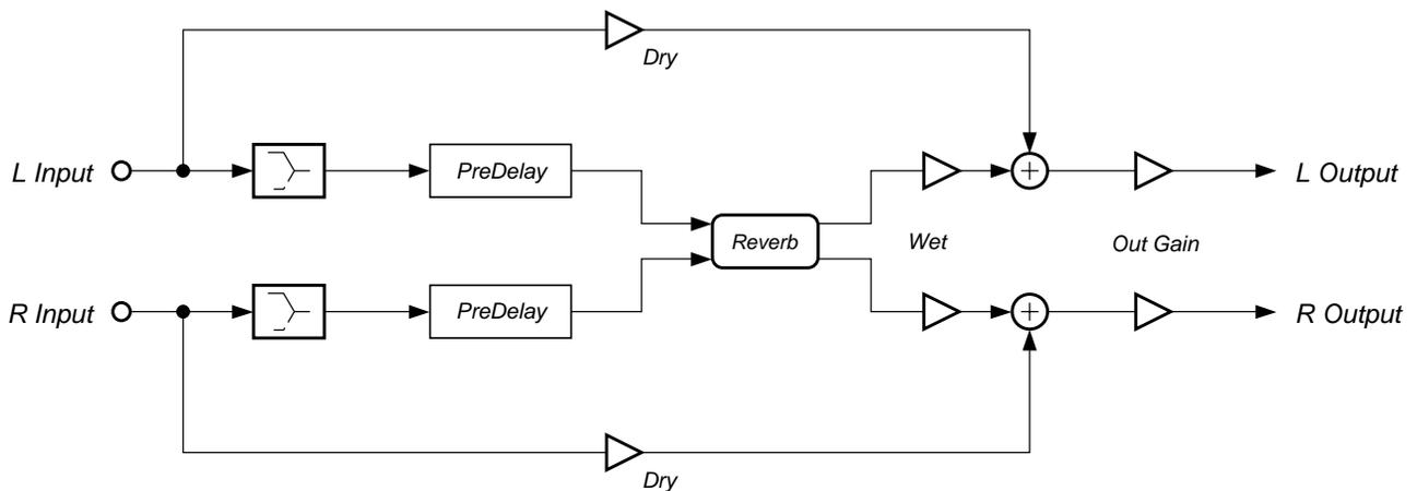
**Figure 10** Simplified block diagram of Panaural Room
