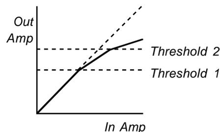
**Figure 97** Two-segment compression characteristic
