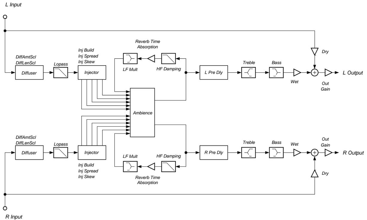
**Figure 9** Signal flow of OmniVerb and OmniPlace
