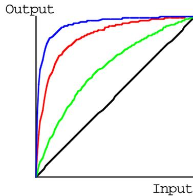
**Figure 69** Input/Output transfer characteristic of soft clipping at various drive settings
