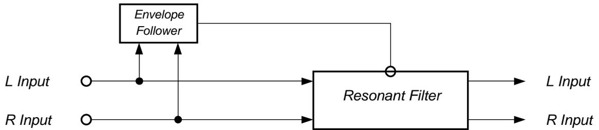
**Figure 105** Block diagram of envelope following filter
