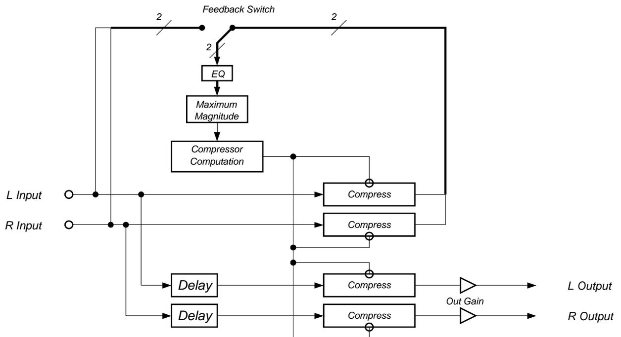
**Figure 86 Compressor with side chain equalization**
