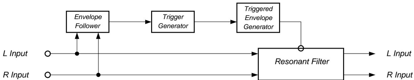
**Figure 107** Block diagram of triggered envelope filter
