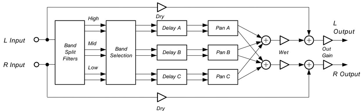
**Figure 29 Stereo 3 Band Delay**
