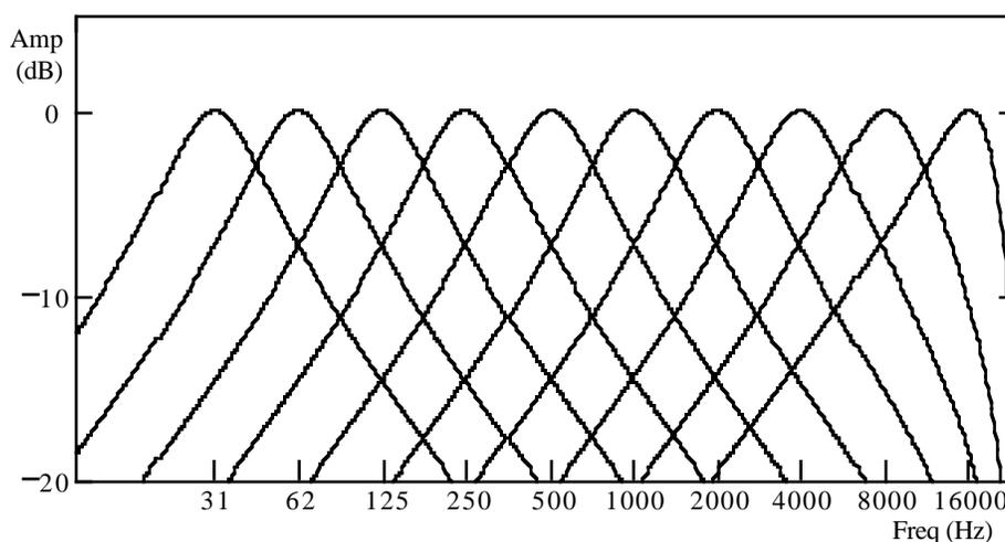
**Figure 102** Filter Response of each Bandpass Filter
