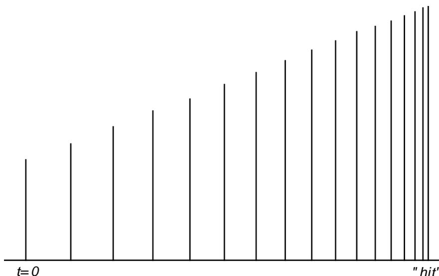
**Figure 19** *Simplified impulse response of Revrse LaserVerb*
