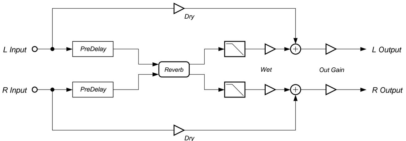
**Figure 11** Simplified block diagram of Stereo Hall
