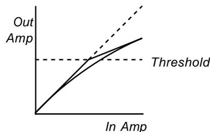
**Figure 13** Soft-Knee compression characteristics
