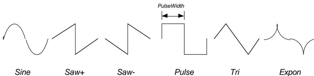
Figure 54 LFO Shapes available for Dual AutoPanner
