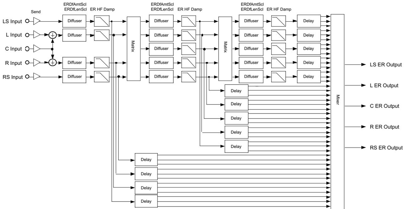
**Figure 152** Early reflection portion of TQ Verb 5.1 and TQ Place 5.1
