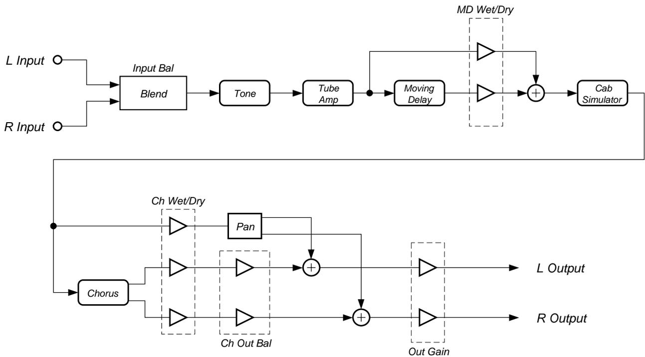
**Figure 83 TubeAmp<MD>Chor with moving delay inserted post-distortion**
