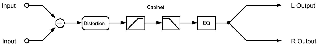
Figure 66 *Block diagram of MonoDistort + EQ*
