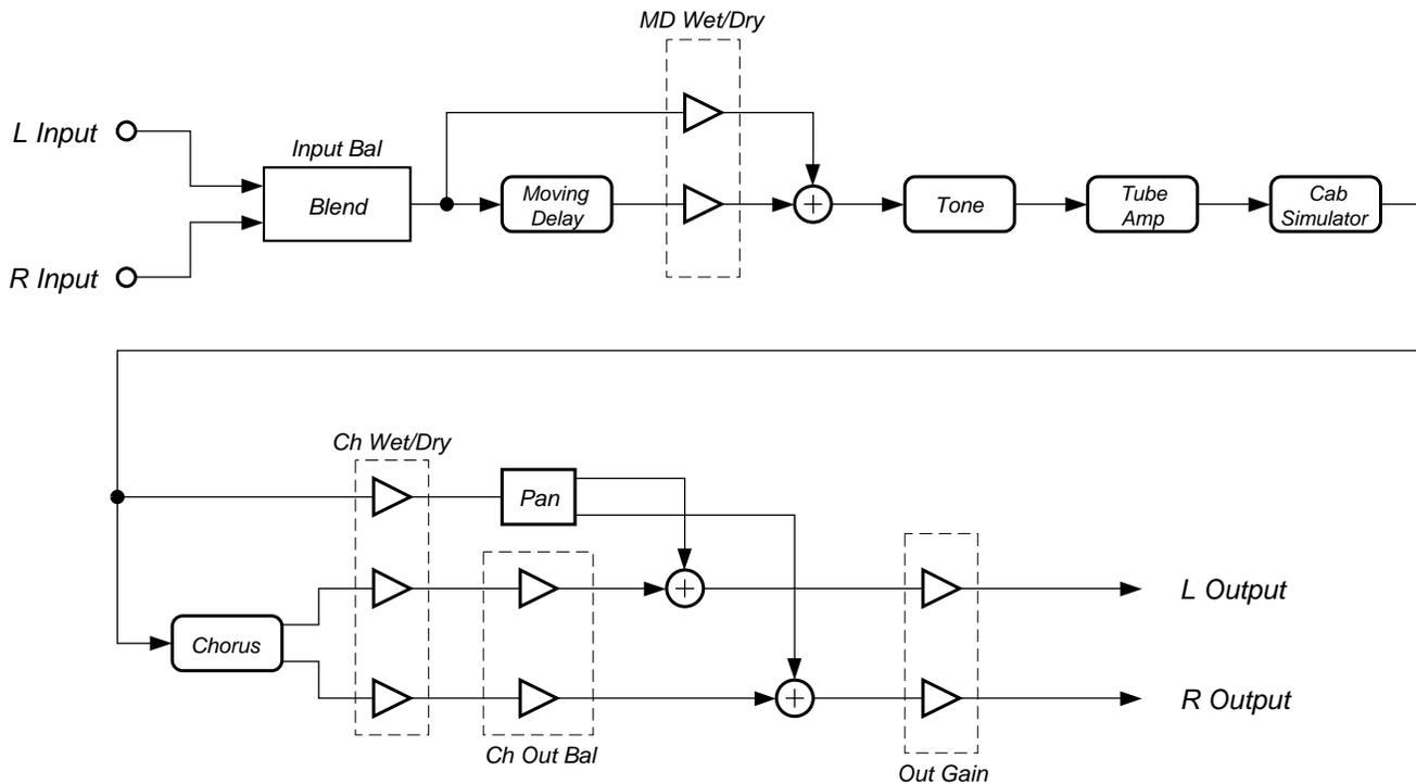
**Figure 82** TubeAmp<>MD>Chor with moving delay inserted pre-distortion
