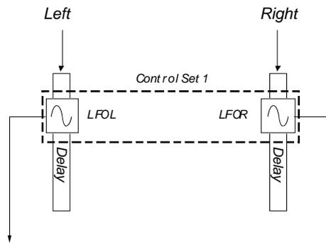
**Figure 148** LFO control in Link1Tap mode
