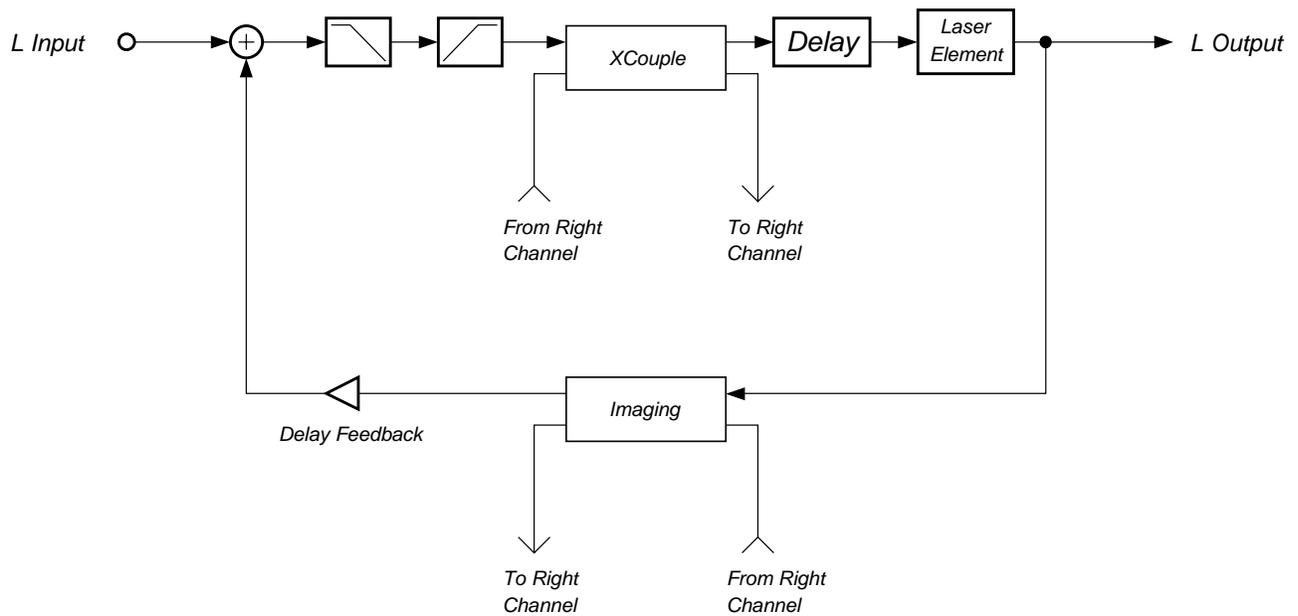
**Figure 150 Laser Delay (left channel)**
