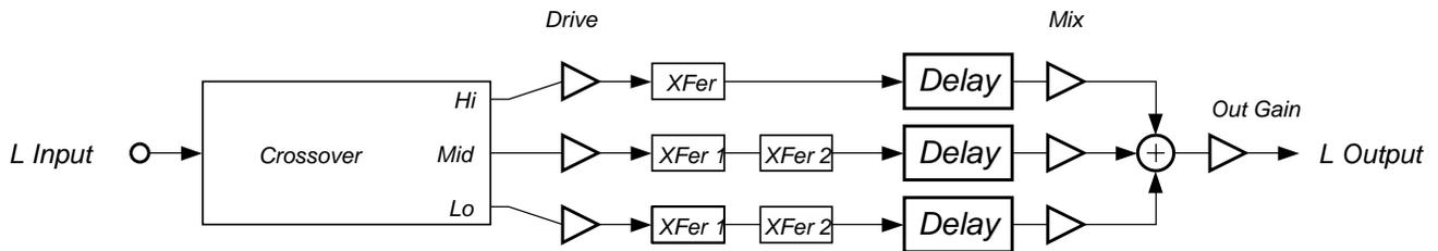
**Figure 113** One channel of 3 Band Enhancer
