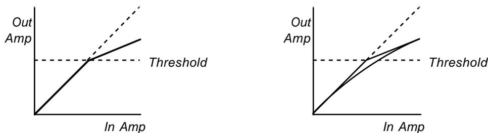
**Figure 156** Hard- and Soft-Knee compression characteristics
