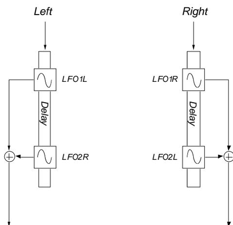
**Figure 146** LFO delay taps in the configurable chorus and flange
