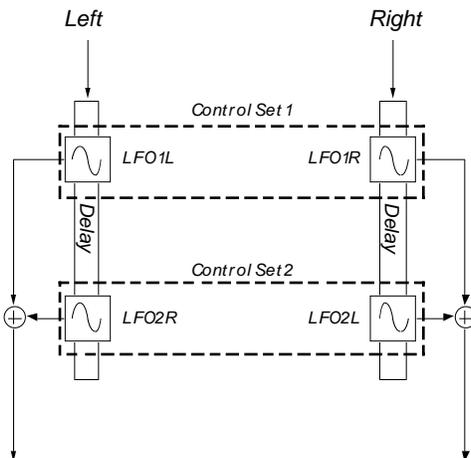
**Figure 149** LFO control in Link2Tap mode
