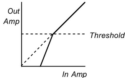
**Figure 98** Expansion transfer characteristic
