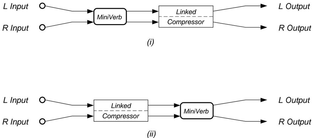
**Figure 14** Simplified block diagrams of **ClascVrb<>Comprs** when set to
