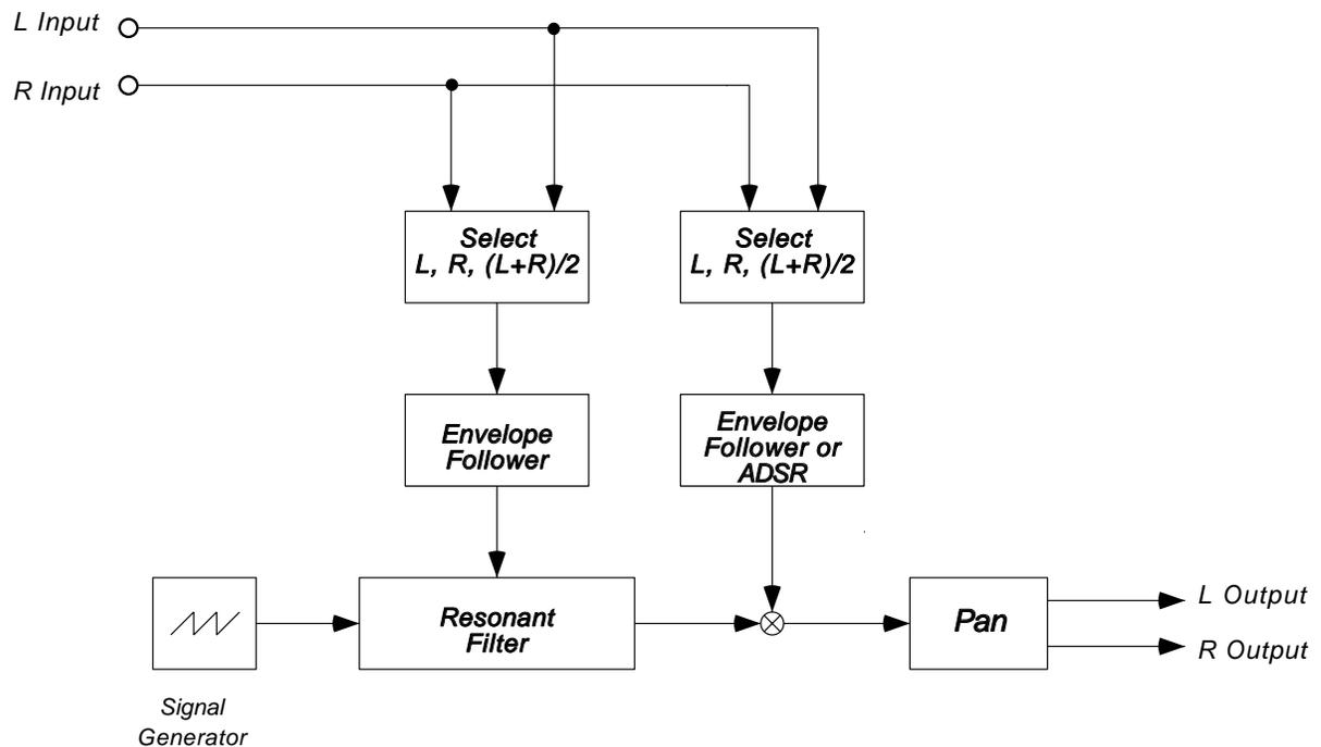
**Figure 139** Signal flow of stereo ADSR Synth and Env Synth
