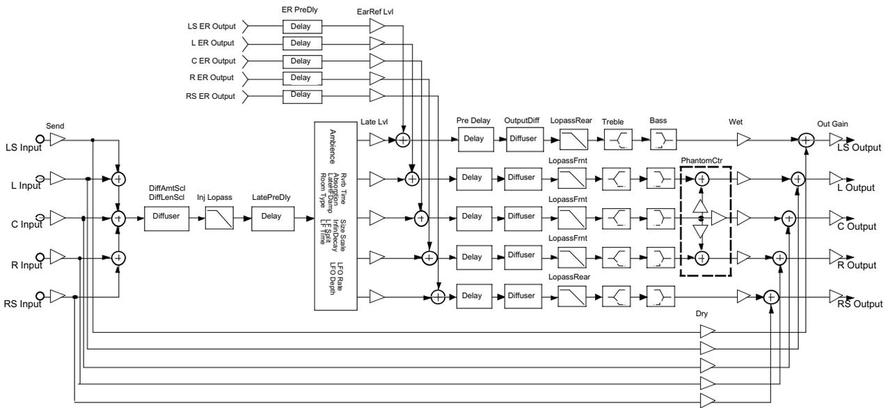
**Figure 153** Signal flow of OmniVerb 5.1 and OmniPlace 5.1
