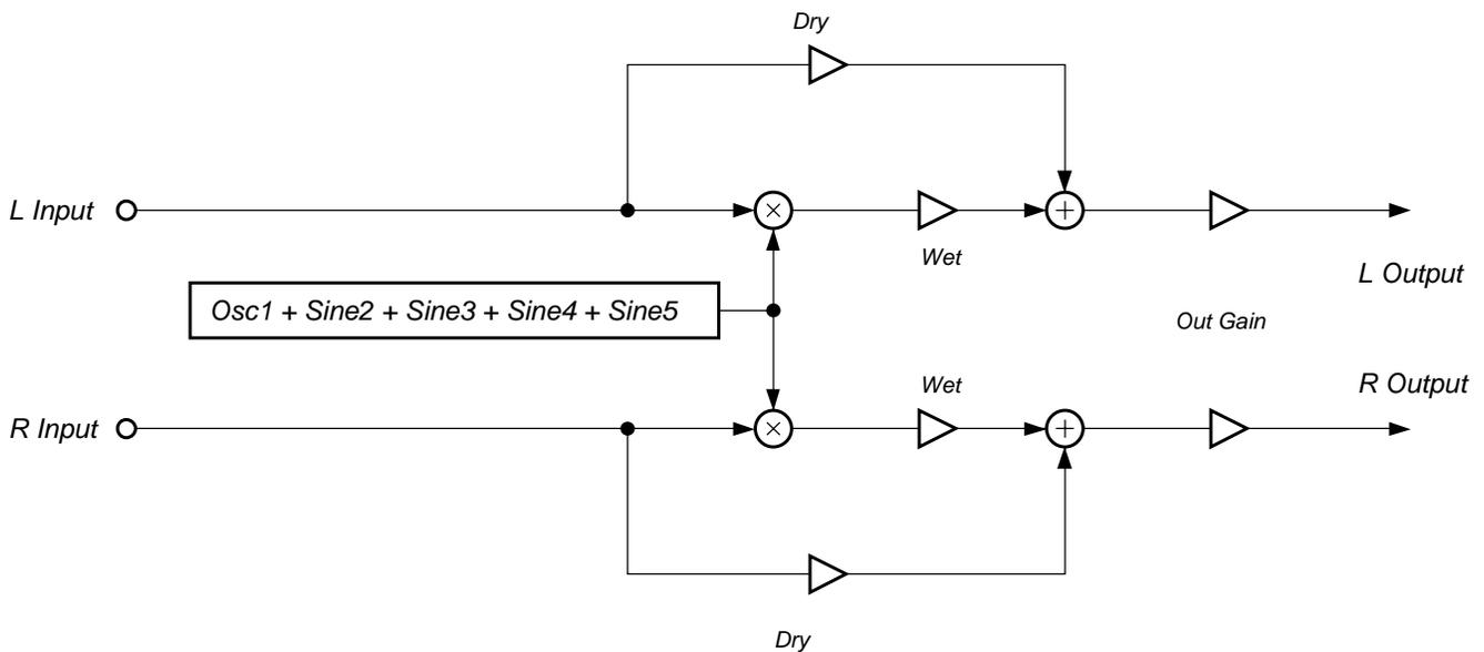
**Figure 121** *Osc mode ring modulator*
