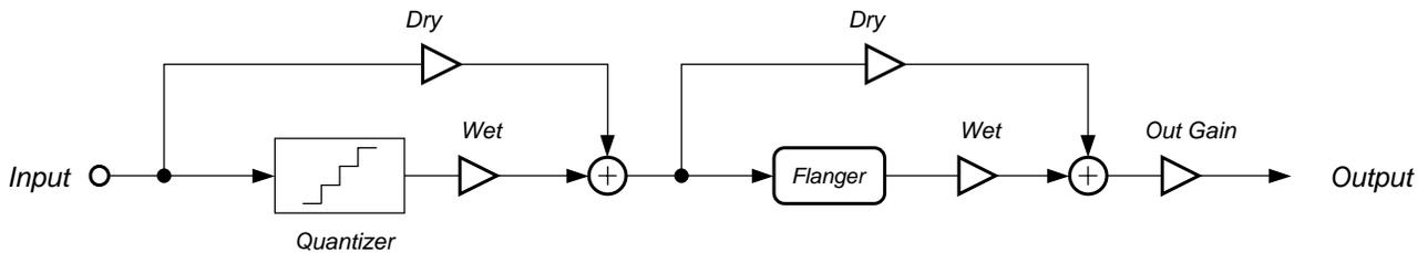
**Figure 75** Block diagram of one channel of *Quantize+Flange*
