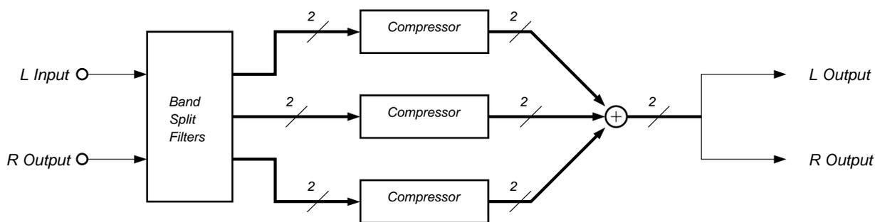
**Figure 92** A three-band compressor
