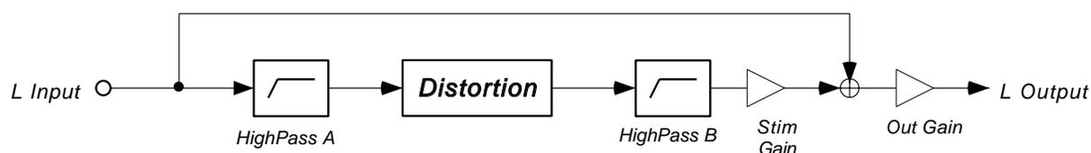
**Figure 114** One channel of high-frequency stimulation
