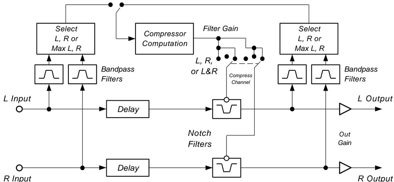
**Figure 90** Band Compress block diagram
