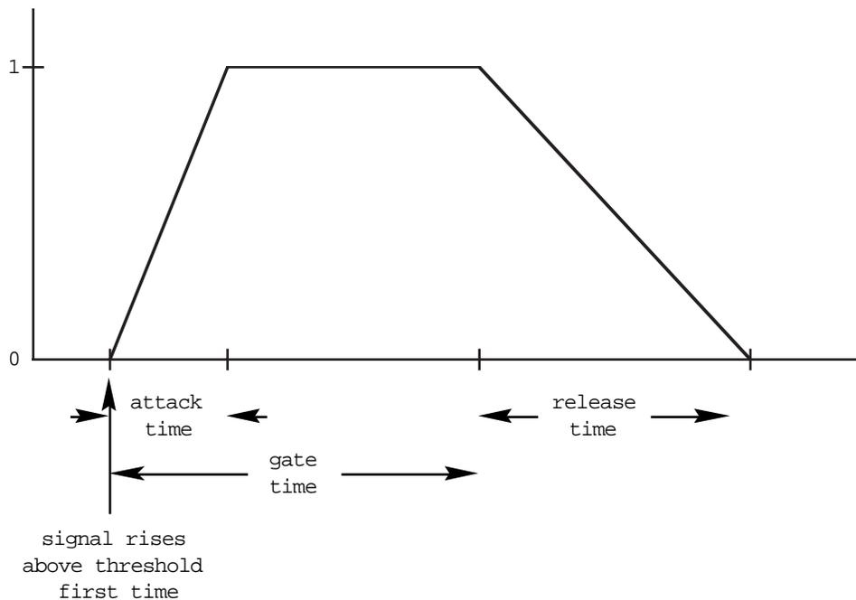
**Figure 101** Gate w/SC EQ signal envelope when Retrigger is Off
