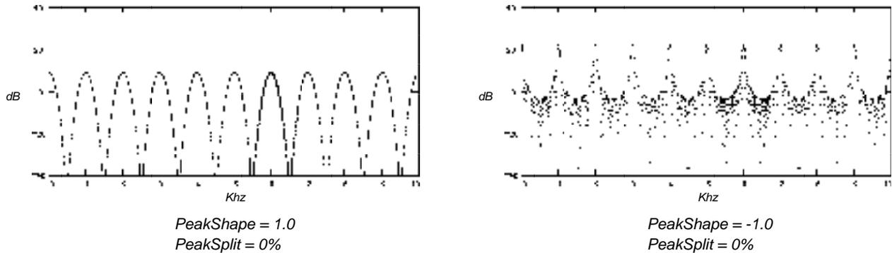
**Figure 144** Response of Pitcher with different PkShape settings
