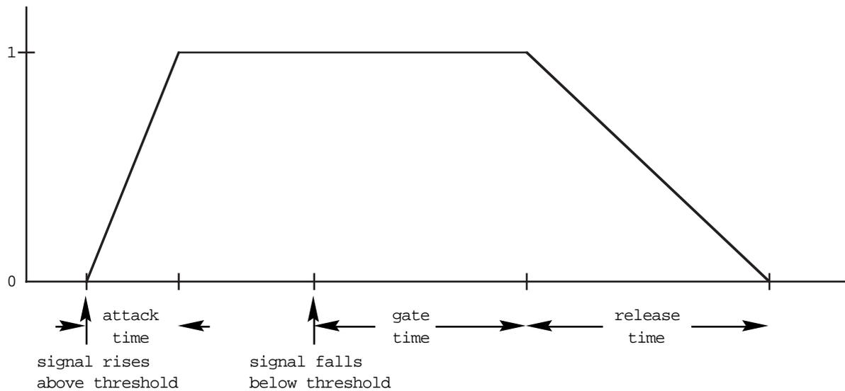
**Figure 100** Signal envelope for Gate and Gate w/SC EQ when Retrigger is On
