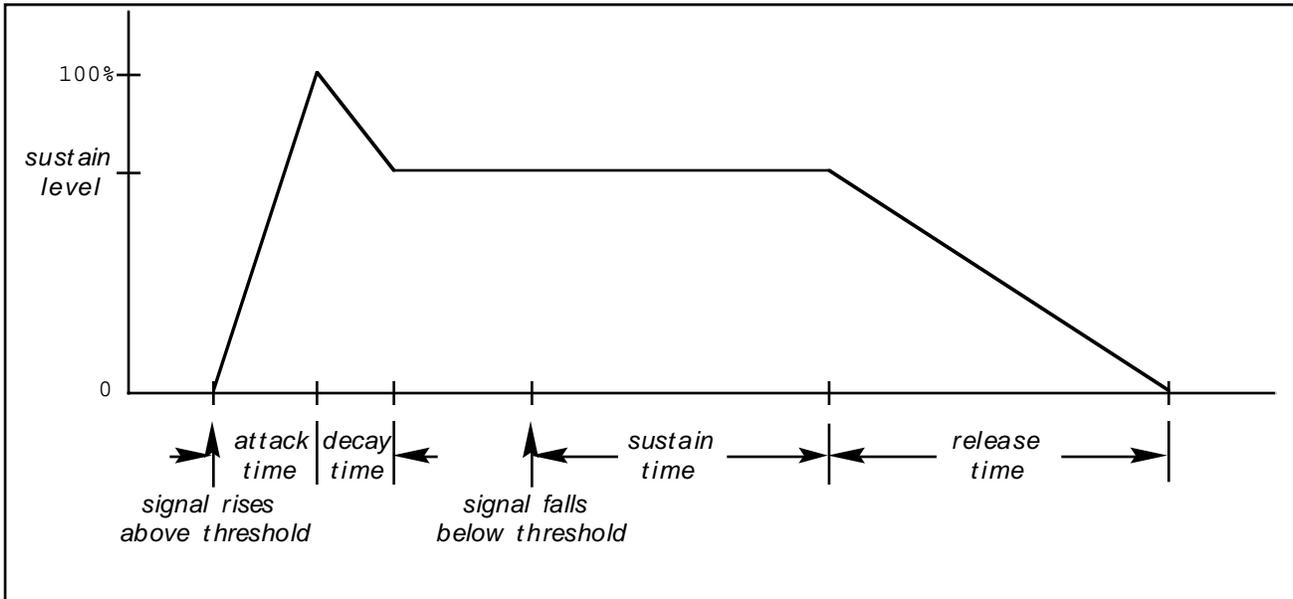
**Figure 141**     **ADSR amplitude control**
