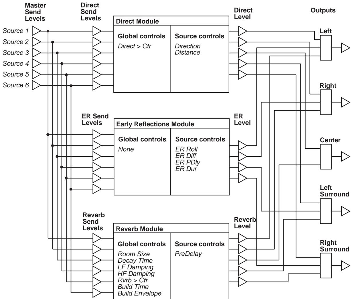
**Figure 155** Simplified block diagram of Surround
