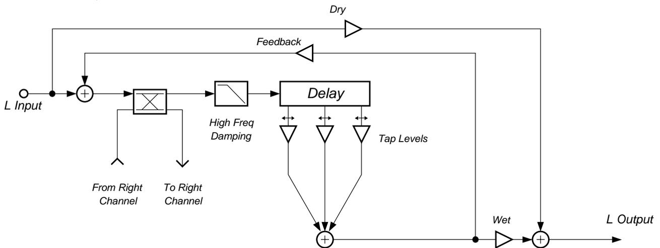
**Figure 34**     Block diagram of left channel of Chorus 2 (right channel is the same)
