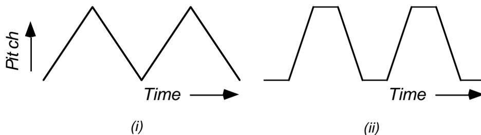
**Figure 39** Pitch envelopes (i) Triangle and (ii) Trapzoid
