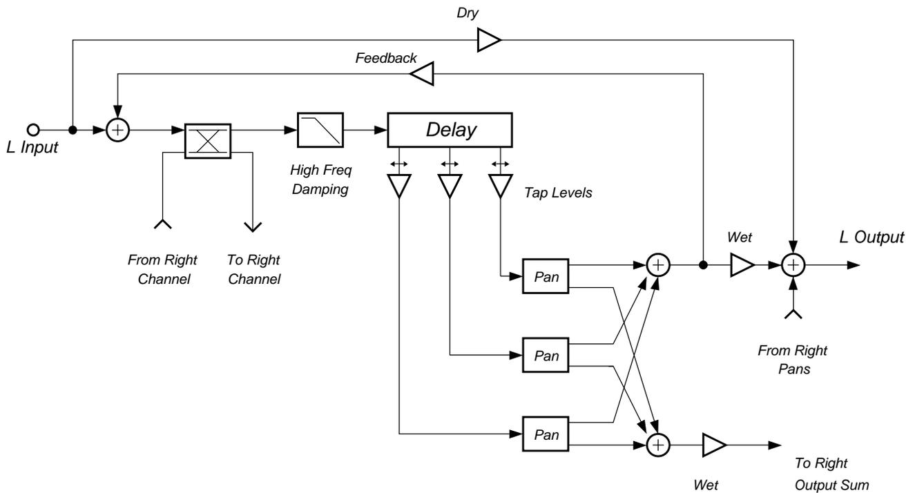
**Figure 35** Block diagram of left channel of Dual Chorus 2 (right channel is similar)
