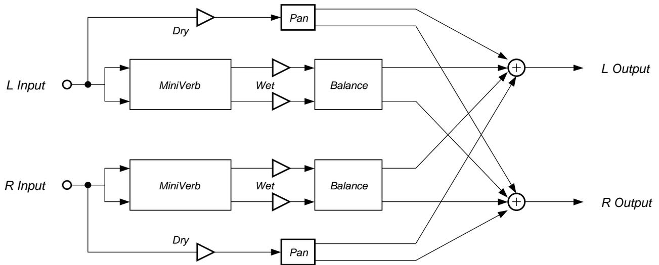
**Figure 2** Simplified Block Diagram of Dual MiniVerb
