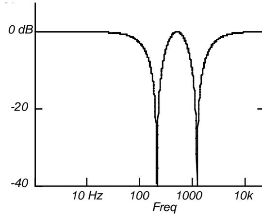
**Figure 45** Response of LFO Phaser Twin with Wet/Dry set to 100%.
