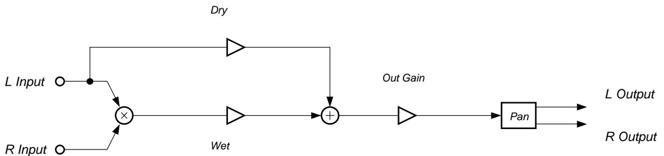
**Figure 120** *L \* R mode ring modulator*
