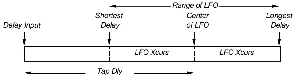
**Figure 43** Delay for a single LFO
