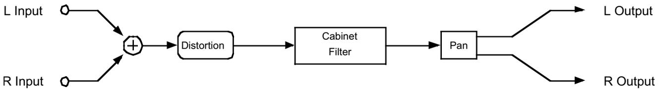
**Figure 68** Block diagram of MonoDistort+Cab
