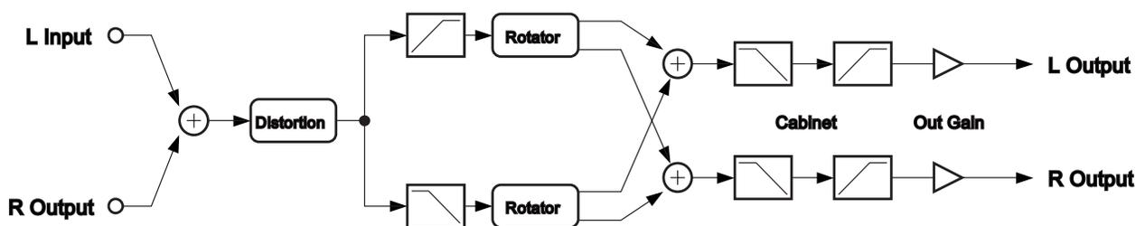
**Figure 61** *Distort + Rotary*
