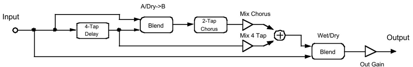
Figure 142 An example of routing using Chorus+4Tap
