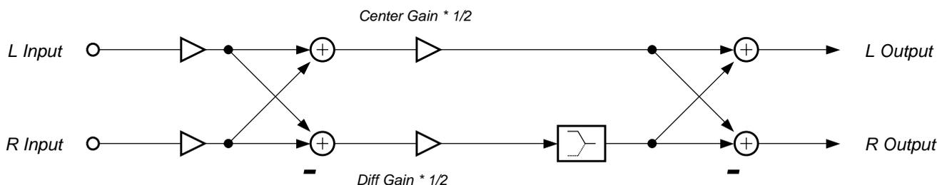
**Figure 55** Block diagram of Stereo Image algorithm
