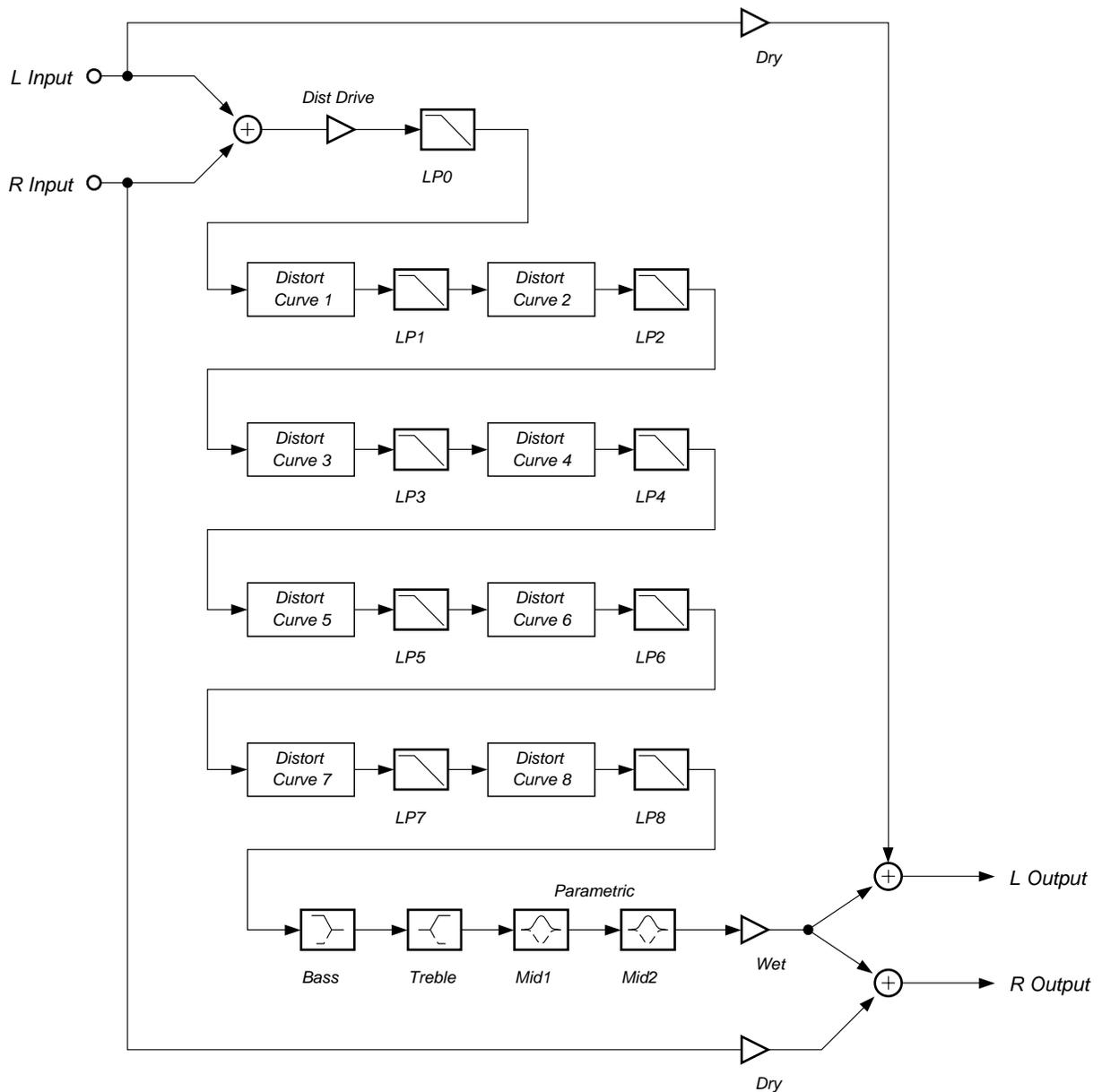
Figure 70 Block diagram of PolyDistort + EQ
