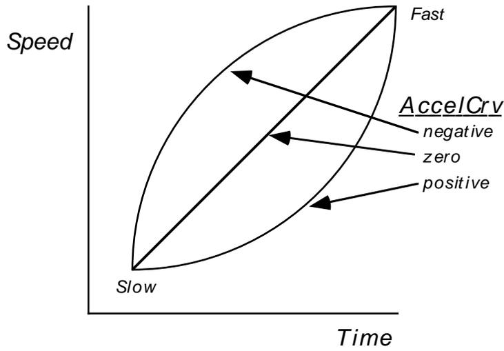
**Figure 60** Effect of acceleration curve on speed
