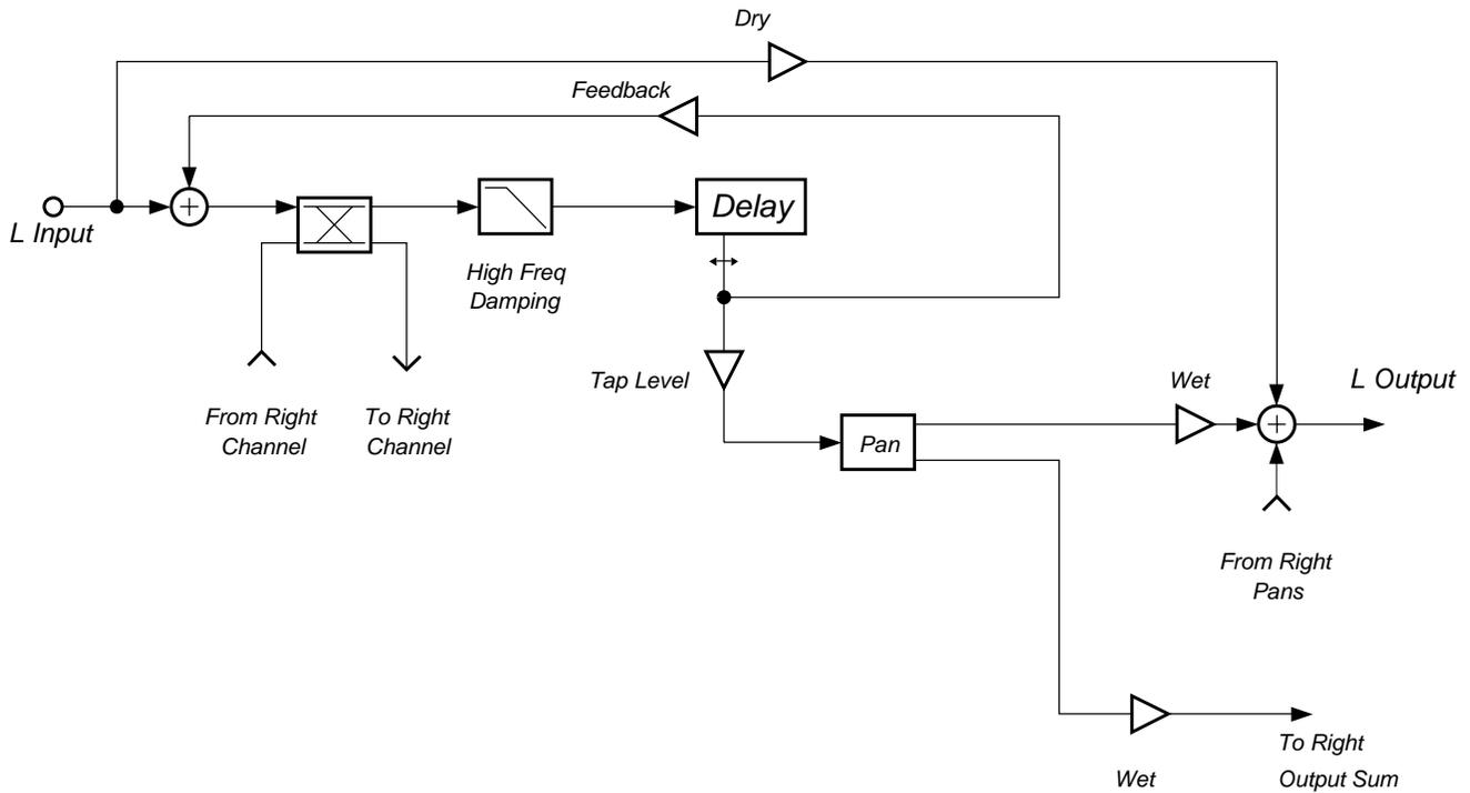
**Figure 37** Block diagram of left channel of Dual Chorus 1 (right channel is similar)
