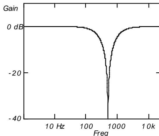
**Figure 115** *Tone Suppressor filtering at full expansion*
