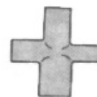
Plug Wrench (You will use this tool when checking the plug or assembling.)
