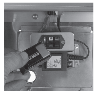
4. Insert and/or replace a new 9V battery
