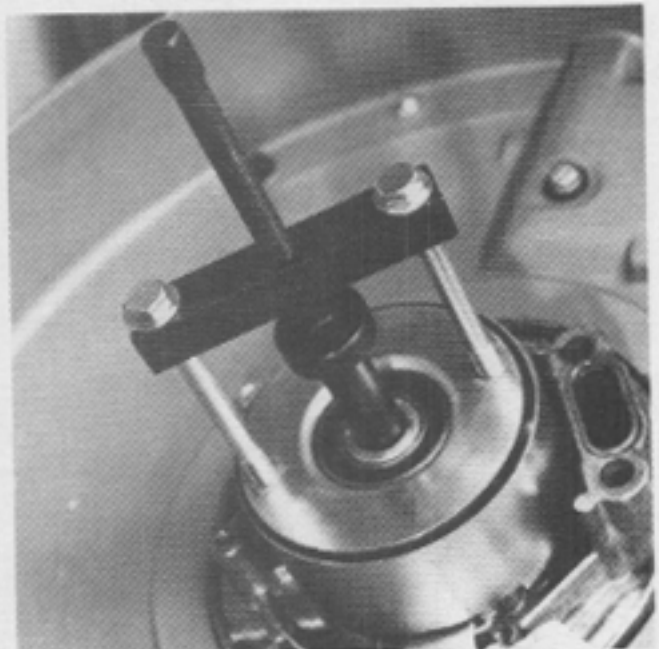
USED TO PULL BRAKE CLUTCH ASSEMBLY.
