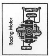
Motors with insufficient or without capacitors can damage your speed control. Therefor you definitely should solder the included capacitors to your motor as shown in the picture.
