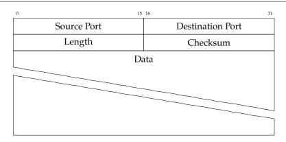
Figure 22.7: Structure of a UDP datagram
