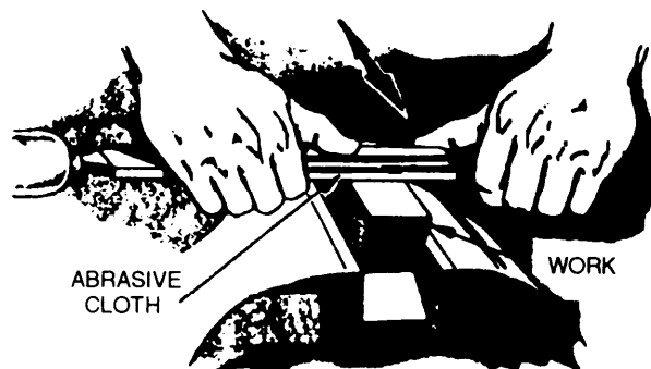
D. POLISHING METAL WITH ABRASIVE CLOTH WRAPPED AROUND A FILE
