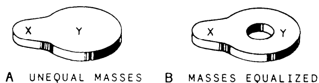
Figure 15-20.—Design of a cam. A. Unequal masses not satisfactory for heat treatment. B. Equalized masses satisfactory for heat treatment.
