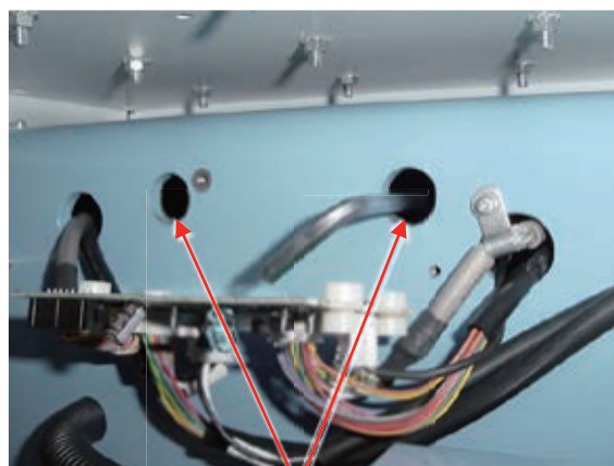
Screw for needle bar change unit inside the beam.
