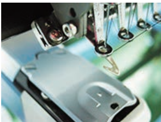
Positional relationship between pressure foot and holder (lower)
