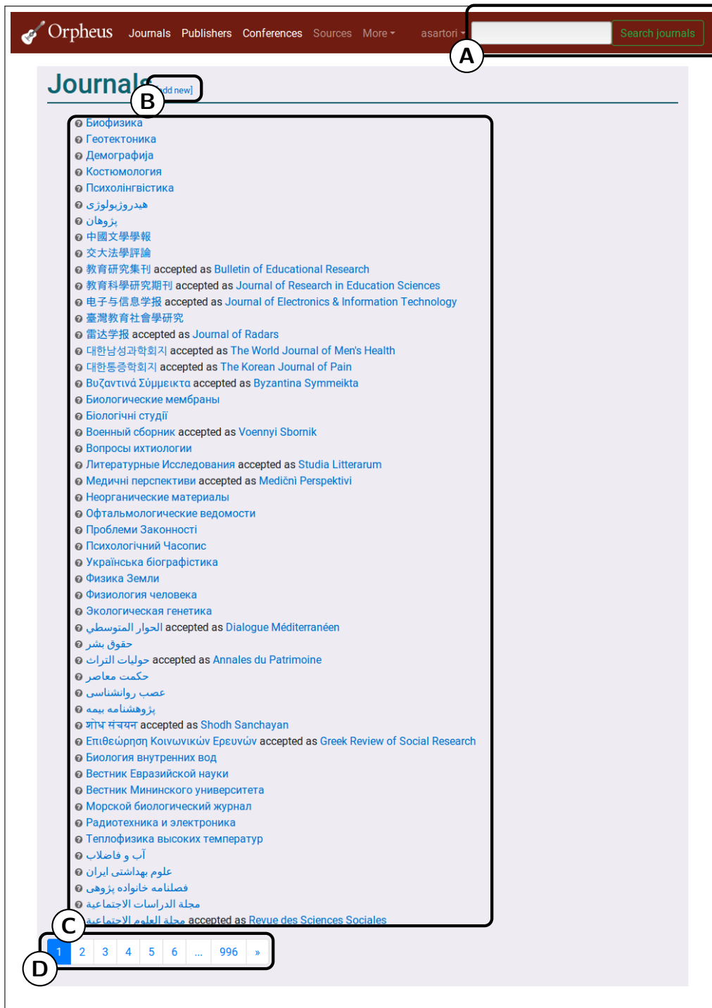
Figure 2: Elements of an Orpheus list view . A , search box; B , “add new” action button; C , list of entries (journals in this case), showing up to 50 records; D , paginator.
