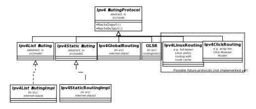
Figure 29.2: Ipv4Routing specialization
