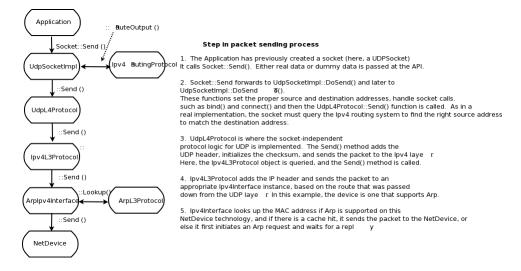
Figure 26.1: Send path of a packet.
