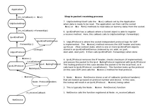
Figure 26.2: Receive path of a packet.
