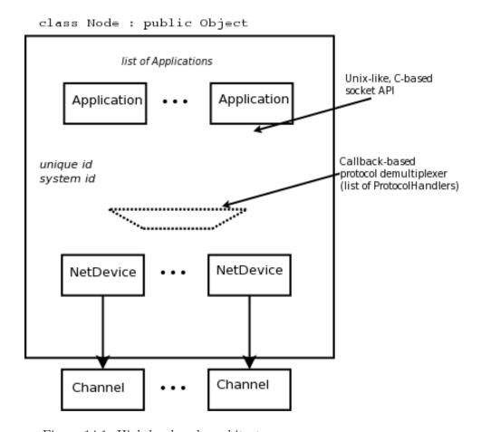
Figure 14.1: High-level node architecture.
