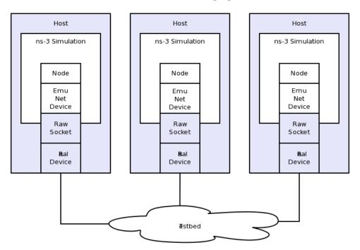
Figure 22.1: Example Implementation of Testbed Emulation.
