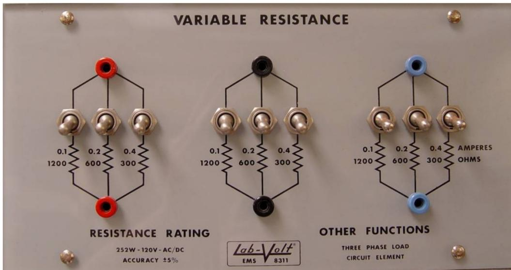
Note: the switch is ON when it is in the “upper” position. Switches allow connecting resistors in parallel and, therefore, change the equivalent resistance of the circuit (load).
