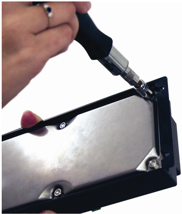
FIGURE 1.10-2. Use a 3/8" socket wrench to remove CR800 canister from wiring panel.
