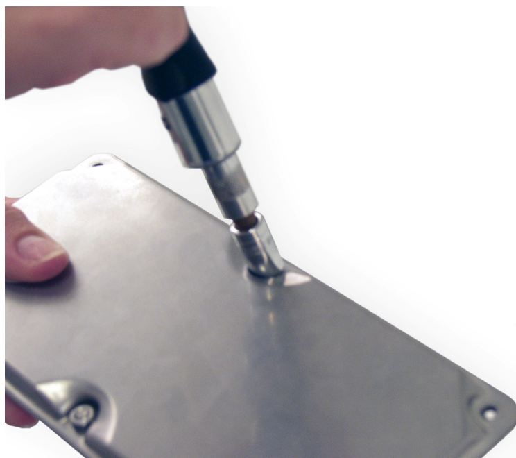
FIGURE 1.10-4. Use socket wrench to disassemble canister.
