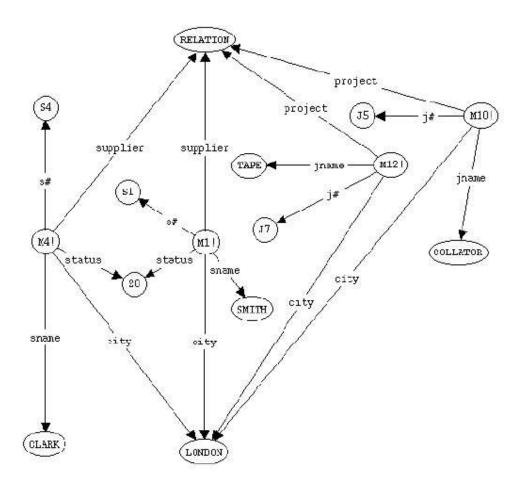
Figure 10.1: Fragment of SNePS network for the Supplier-Part-Project Database
