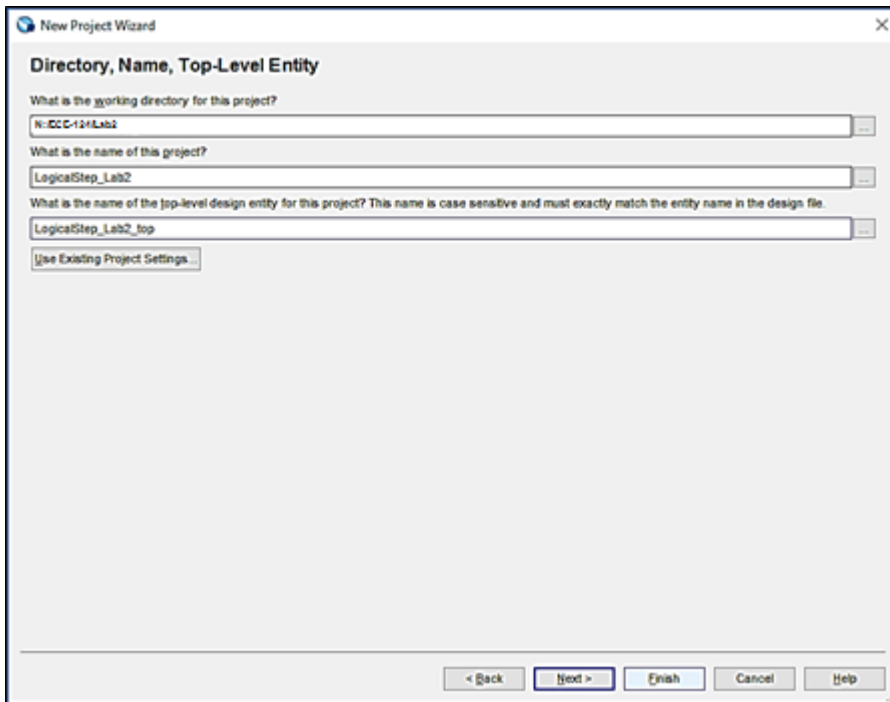
Figure 50 Lab2: FPGA Project Setup
