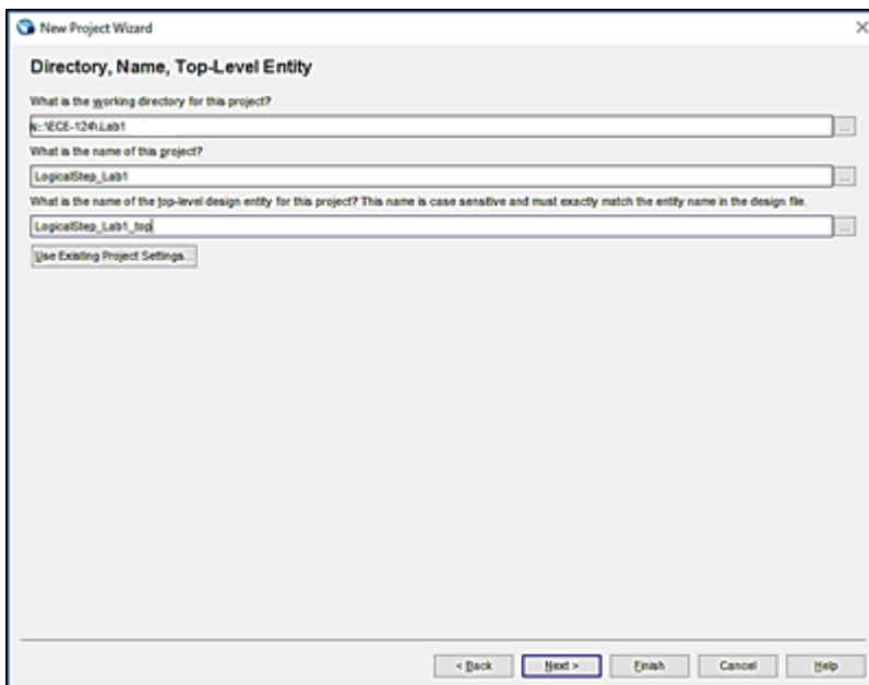
Figure 5 Lab1: FPGA Project Setup
