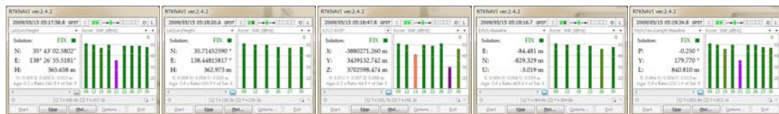
Figure 3.2-17 Solution Status Display of RTKNAVI
