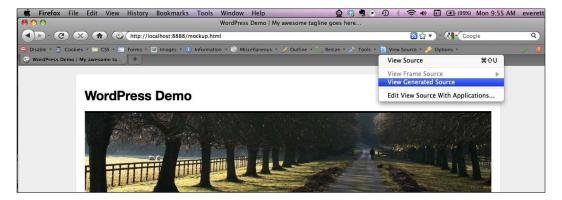
When we use the Web Developer Toolbar and **View Source** | **View Generated Source**, we can see our text both in the head and where we inserted it in the target div. We highly recommend using this plugin to check your work as you manipulate pages using JavaScript.
