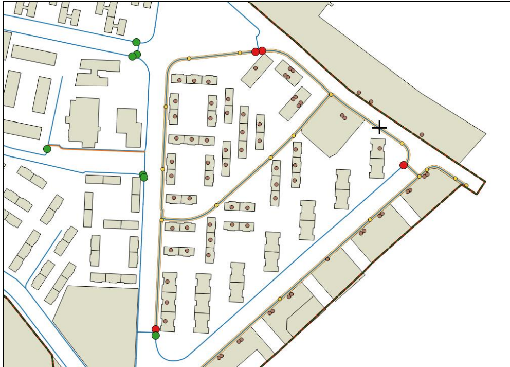
Image 31: View of the map showing the results of the mincut process. The symbology shows the valves to close, as well as arcs, nodes and connects affected by it.
