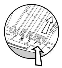
**2.** On the back of the phone, remove the key located behind the hookswitch and reposition it so that the end tab (at a  $45^{0}$  angle) is facing up.
