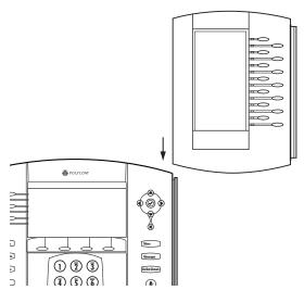
**3.** Connect the base stand by aligning the two protrusions on the stand to the holes on the back of the Backlit Expansion Module and snap it into place.
