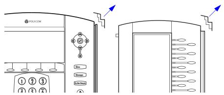
**2.** Align the SoundPoint IP Backlit Expansion Module at the top of the groove lines on the SoundPoint IP 650 phone and slide it downwards until it clicks into position.
