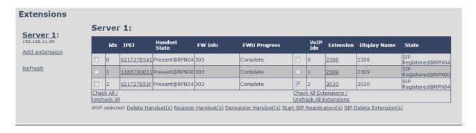
**STEP 8** Confirm the SIP registration by SIP State in right column.
