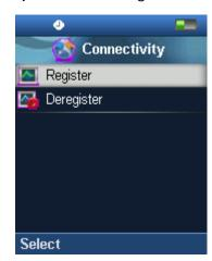
c) Type in the "AC code" and press "OK" to start the registration. The default AC code is "0000".
