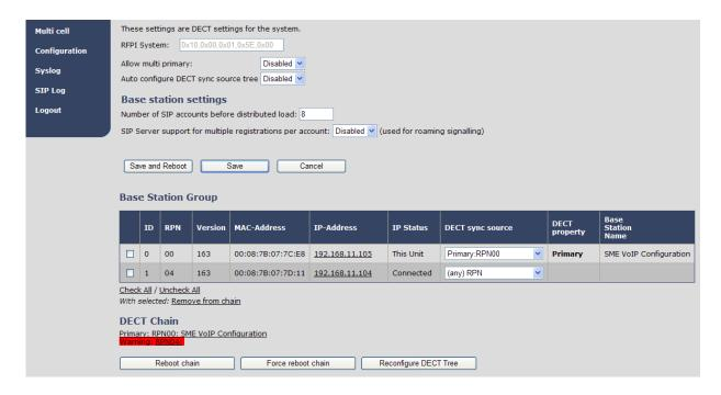
STEP 13 On the Multi-cell settings page, scroll to the DECT system settings and Enable or Disable the "Auto configure DECT sync option source tree" (See description in the table below). The DECT system RFPI parameter is computed by the system (It's often greyed in a multi-cell system configuration).
