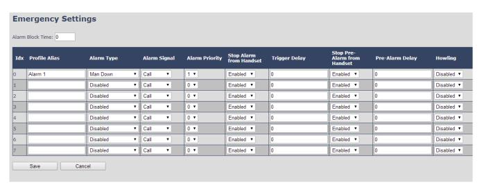
All configuration of the handset Emergency Settings is done from the base station. The concept is that on the "Emergency Settings" page on the web server, eight different alarm profiles can be configured. Afterwards for each handset, it can be selected which of the configured alarm profiles, the given handset shall subscribe to. When this is done the selected alarm profiles are sent to the handset. See section 5.3.2.3 Multiline: Edit handset
