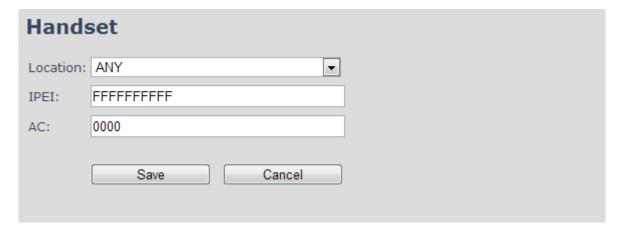
**STEP 5** Enter the IPEI of handset which must register to this particular extension and press "Save"
