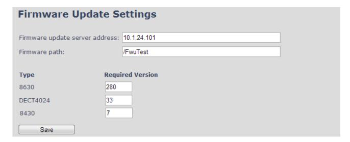
**NOTE:** To disable handset/repeater firmware process type version 0 in the required version field, followed by the save button. It is recommended to use version 0 after all units are upgraded.
