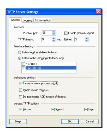
• Configure the relevant TFTP virtual folder in the server. The TFTP virtual folder is the file folder, visible for TFTP clients under a certain name. You can set security settings separately for every virtual TFTP folder. Next, set rights to access TFTP folders according to the relevant clients.
