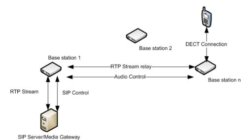
After handover to BS n the handset is located at BS n, and the RTP stream is relayed via BS 1.
