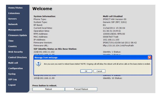
This will trigger **Are you sure you want to reboot base station?** window. Click **OK** button on this window. A successful restart of the base stations will lead to a display of the page: **Gateway has been reset**.
