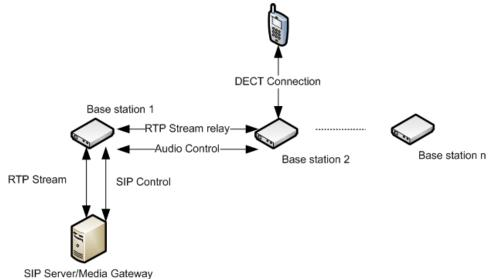
Stage 2: After handover to BS 2, the HS is located at BS 2, and the RTP stream is relayed via BS 1.
