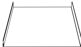
1 1/2" SSR 24 Gauge Standing Seam Roofing
