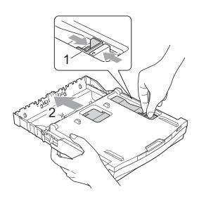
Press and slide the paper side guides (1) and paper length guide (2) to fit the paper size.
