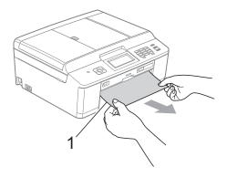
4 Lift the Jam Clear flap, and remove the jammed paper.
