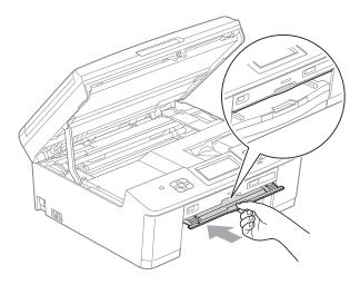
7 Using both hands, grasp the plastic tabs on both sides of the machine and gently close the scanner cover.
