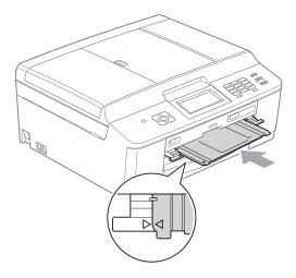
6 After the disc has finished printing, close the Disc Guide and store the Disc Tray back in the scanner cover.
