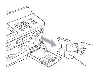
Open the new ink cartridge bag for the colour shown on the LCD, and then take out the ink cartridge. 4 Turn the green release lever on the orange protective packing (1) clockwise until it clicks to release the vacuum seal. Then remove the orange protective packing as shown.
