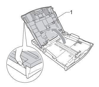
With both hands, gently press and slide the paper side guides (1) and then the paper length guide (2) to fit the paper size.
