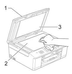
In the ADF unit, clean the white bar (1) and the glass strip (2) with a lint-free cloth moistened with a non-flammable glass cleaner.
