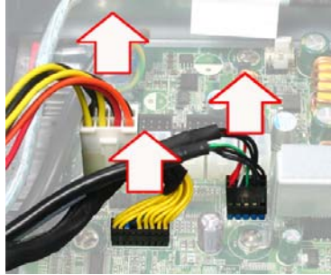
Front right to left: PW6 cable, Fan Tach Connector cable and USB cable
