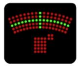
To get a sense of what you'll see, let's look at the whole LED matrix with all of the LEDs illuminated. The green arc is the "in tune" line when in the polyphonic mode. The vertical array of green LEDs is the needle pointer in the mono mode when you're perfectly in tune. The small group of four red LEDs is the # (sharp) indicator. It doesn't display flats when tuning, only when adjusting it
