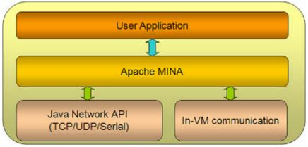
Here, we can see that MINA is the glue between your application (be it a client or a server) and the underlying network layer, which can be based on TCP, UDP, in-VM comunication or even a RS-232C serial protocol for a client.
