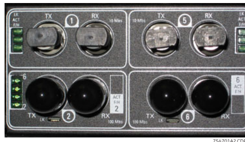
FIGURE 2-1: Example two-Port 10Mb mm fiber ST module & two-Port 100Mb mm fiber ST module
