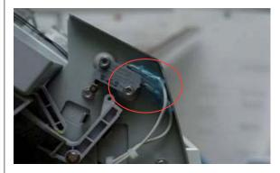
3. Check the Safety Unit's operation. Check the switch is clicked when the Safety Link moves.
