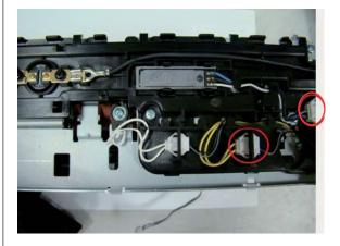
5. Remove the thermistor. Check if the thermistor has curled as shown below. If there is any contamination on the film, clean it.
