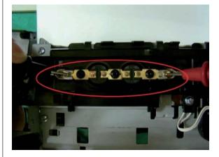
7. Remove the FDB cover. Check if the FDB Triac is short. Check the resistance among 3 legs of both transistors. If it is short, replace the FDB.
