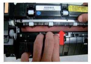
b. Release the both hooks with the tweezers or (-) driver.
