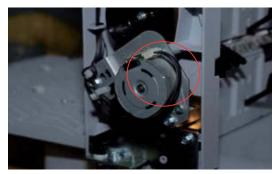
2. Check Lower Diverter Sensor Harness connection.
