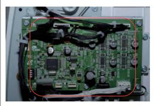
2. Check the Finisher Support Finger Home Sensor's Harness Connection.
