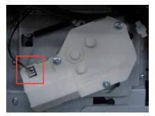
4. Check if the Press D-Cut of the Gear-Lifting is deformed or broken.
