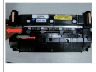
b. Rotate the gear to direction of arrow and check the surface of the Hear roller and Pressure roller. If there is any overheated traces, replace the fuser unit.
