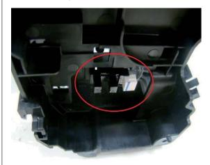
6. Check if the left/right CAM and the ENCORDER are assembled properly.
