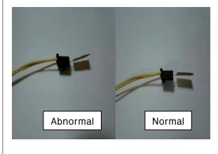
6. Measure the thermostat resistance. Check if the thermostat is opened.
