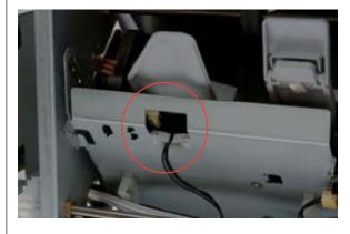
3. Check the Finisher Support Finger Motor's Harness Connection and operation.
