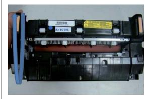
c. Remove the COVER-UPPER. Check if the thermistor harness is connected properly and the thermistor is defective.
