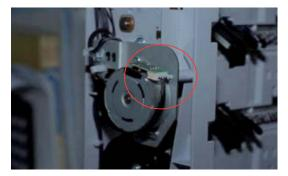
2. Check Upper Diverter Sensor Harness connection.
