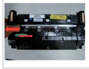
b. Rotate the gear to direction of arrow and check the surface of the Hear roller and Pressure roller. If there is any overheated traces, replace the fuser unit.
