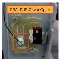
3. If the connection is OK, replace the PBA-SUB Cover Open.
