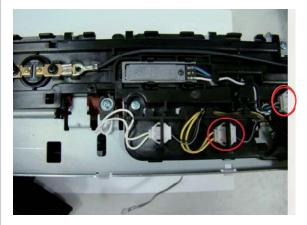
4. Remove the thermistor. Check if the thermistor has curled as shown below. If there is any contamination on the film, clean it.
