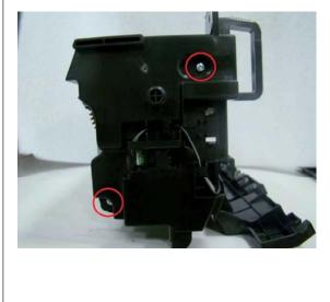
5. Check if the photo sensor connector from the COVER-RIGHT is connected properly.
