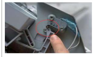
4. Check the Safety Unit's operation using Rear Jogger. The same "switch ON/OFF" operation should be followed.
