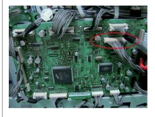
7. Check if the FDB connector is connected properly.
