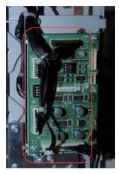
3. Check the Rear Door Switch Harness connection.
