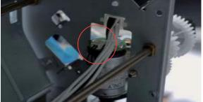
4. Check the Stack Full Sensor Connection and operation.
