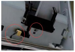
3. Check the Stacker Motor Harness Connection and operation.
