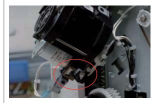
3. Check if staples are stuck in Stapler Head area and damage of Stapler itself.
