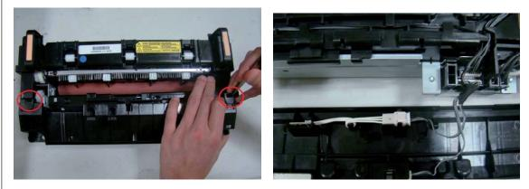
4. Remove the COVER-LEFT after removing 2 screws. Remove the COVER-RIGHT after removing 2 screws.
