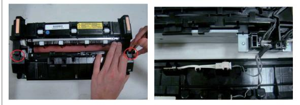
4. Check if the fuser is assembled and fuser connector is connected properly.
