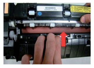
b. Release the both hooks with the tweezers or (-) driver.
