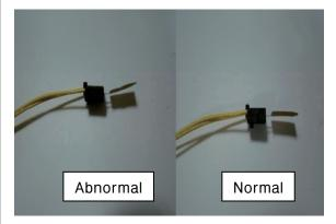
6. Check if the thermistor connector on the engine board is connected properly.
