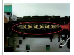
3. Measure the LAMP-HALOGEN resistance value from the center and both sides. Check if it has the continuity.
