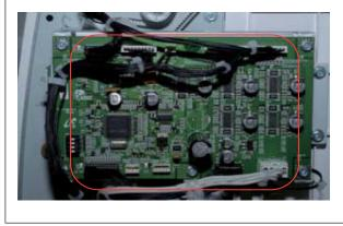
4. Check the Stapler Door Switch Harness Connection.
