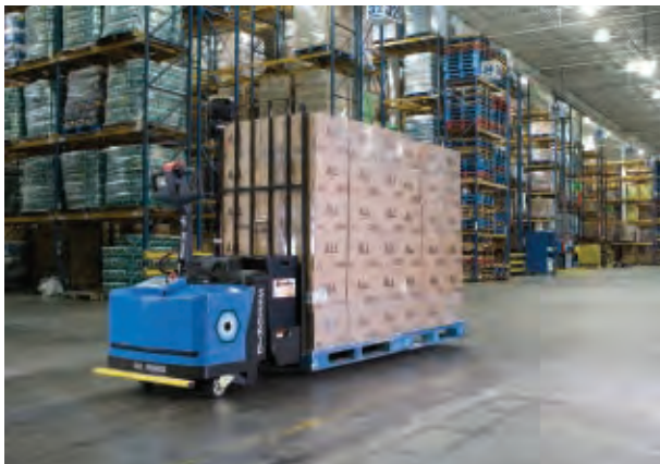
New navigation systems, like image-based navigation from Seegrid, are enabling flexible AGVs that can easily find their way to any spot in a plant or distribution center.
