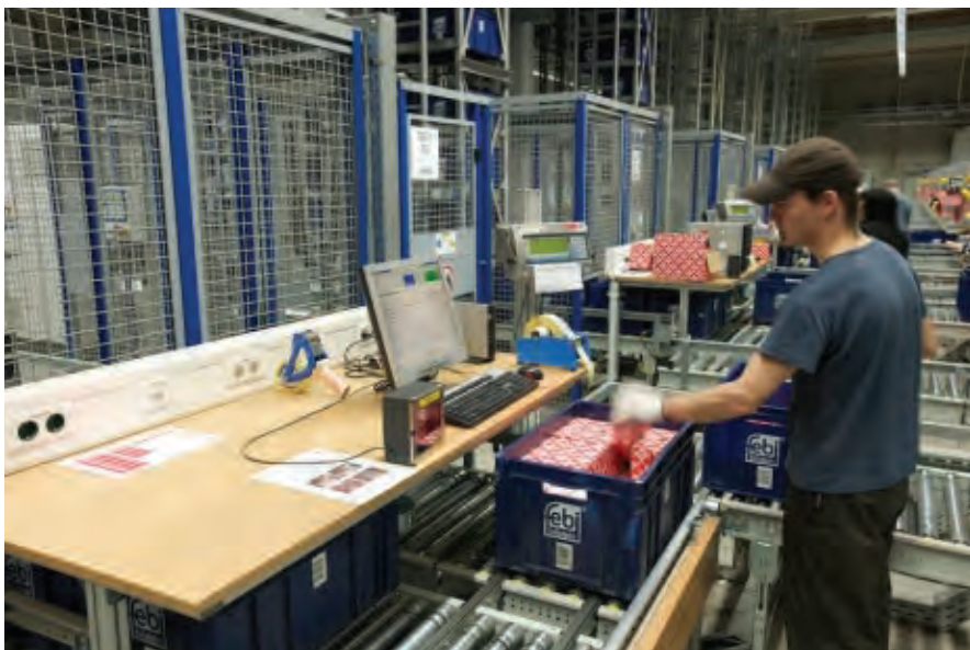
Totes are delivered from the mini-load AS/RS to workstations. Febi employees played a role in the ergonomic design of their work areas.
