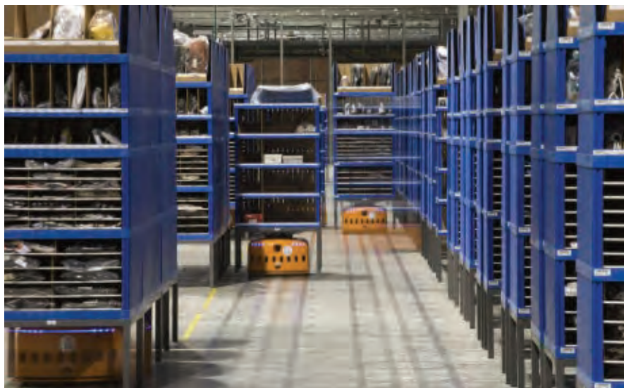
Mobile robots, like this one from Kiva, are taking AGVs into new applications, like goods-to-person order fulfillment.
