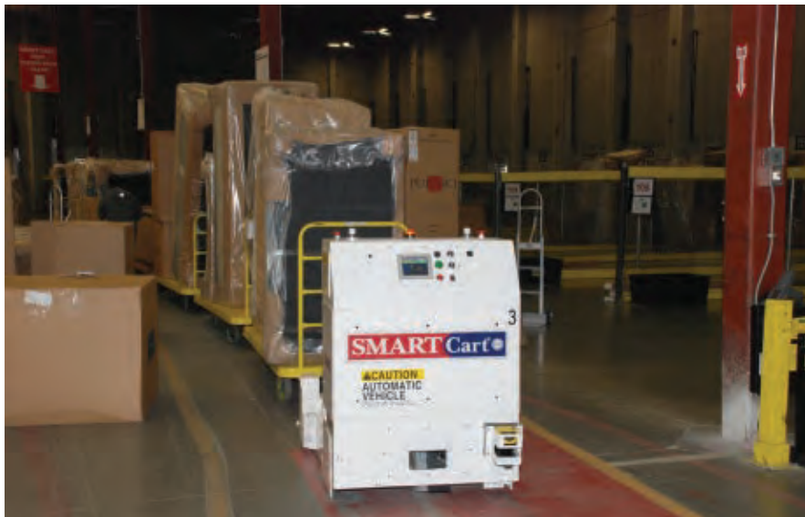
First introduced at ProMat 2005, automatic guided carts have proved themselves in lineside delivery of parts and as an alternative to fixed path assembly lines for many manufacturers.
