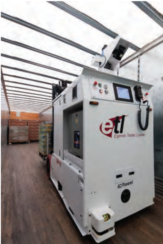
Automatic trailer loading AGVs, or ATLS, can now load and unload trailers and interface with deep-lane pushback rack systems.
